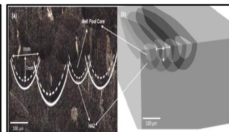
**Figure 3.** Optical and FE Simulation Validation of Melt pool
