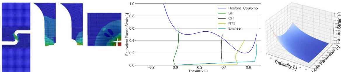
Figure 2 – FE mesh of the coupons (left), Calibrated Hosford-Coulomb model for shell element (middle), Calibrated Hosford-Coulomb model for solid element (right)
