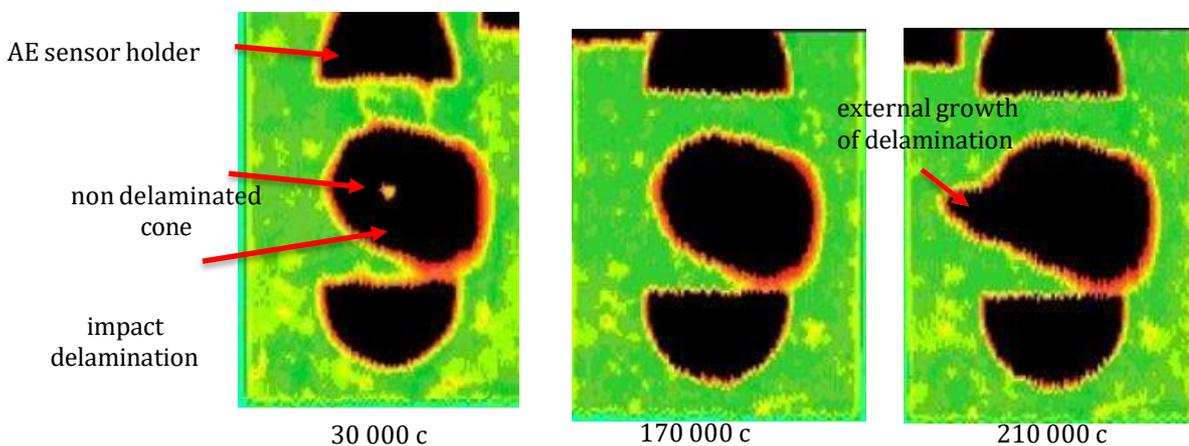
**Figure 1** – C-scan image of delamination at different stages during the fatigue test, showing growth into the non-delaminated cone
