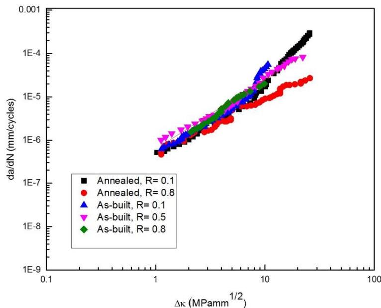
**Figure 3-** Hartman and Schijve representation of FCGR of Ti-6Al-4V tested at different R ratios [1]
