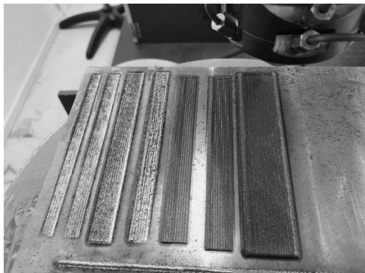
**Figure 1** - Example of preparation of the bi-material interface made by the laser cladded protective layer on structural steel.
