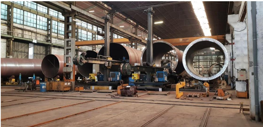
*Figure 1 – Tubular steel towers sections. Courtesy of Tegopi.*
