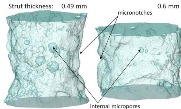
**Figure 1** – Concerned additive manufactured Ti–6Al–4V lattice struts
