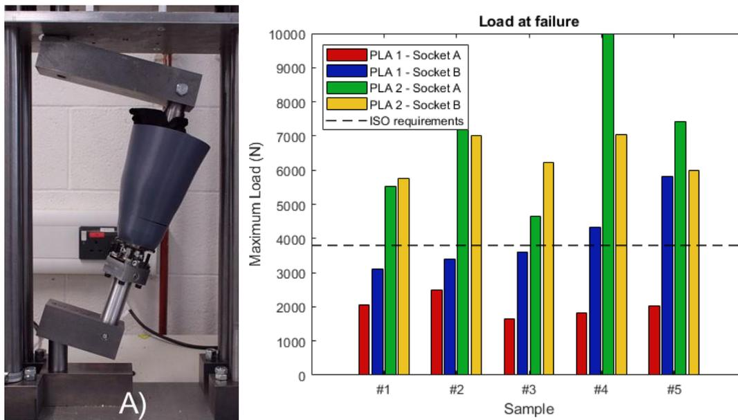
**Figure 1** – A) Ultimate-strength testing configuration. B) Maximum load at failure for two different socket designs printed with two different materials.
