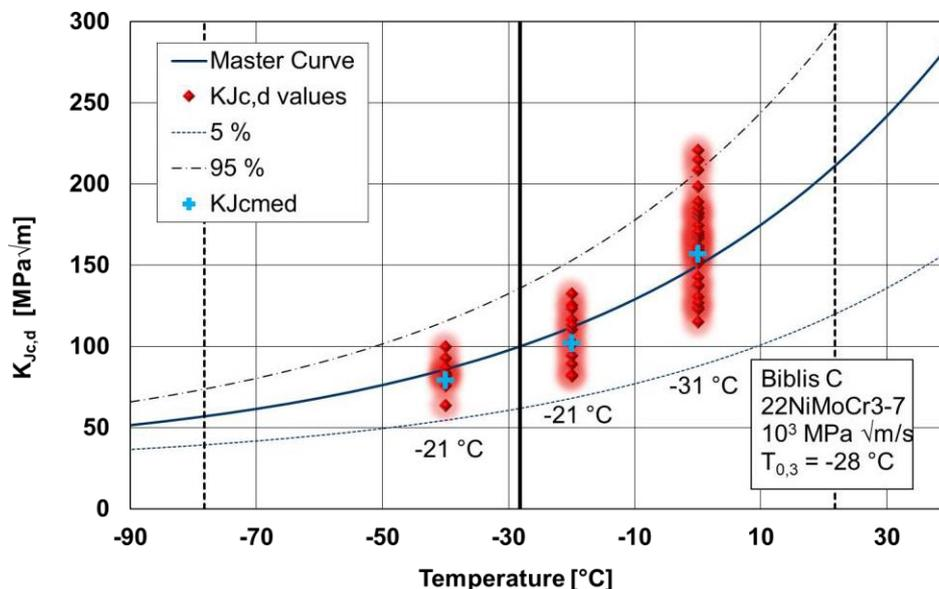
**Figure 1** - Comparison between multi-temperature Master Curve evaluation and single-temperature Master Curve evaluation at different test temperatures for  $10^3$   $\text{MPa}\sqrt{\text{m/s}}$ , 22NiMoCr3-7 (Biblis C)
