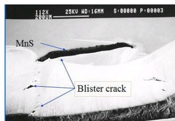
**Fig. 2b. Blister (Laboratory Test) in X-65 linepipe Steel.**
