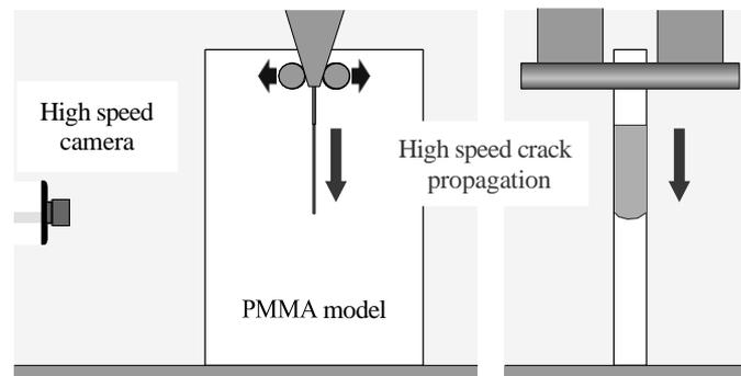
*Figure 1 – Experimental setup for crack arrest test using PMMA.*
