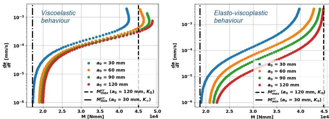
**Figure 1** – Crack propagation rate as function of the critical applied moment
