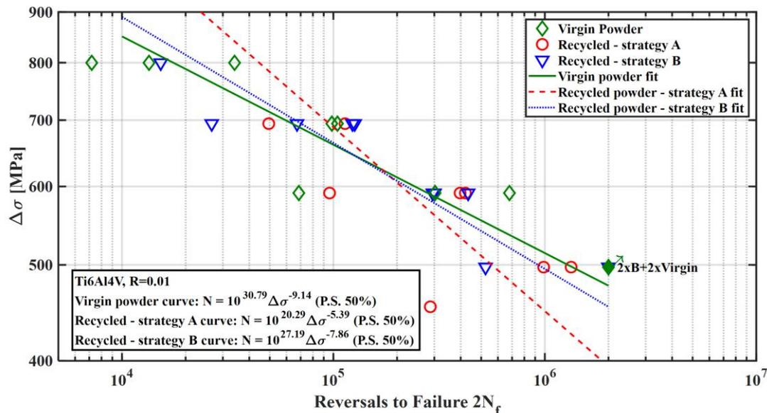
**Figure 1** – Stress vs Cycles to failure for Ti6Al4V AM specimens realized using virgin and recycled material feedstock
