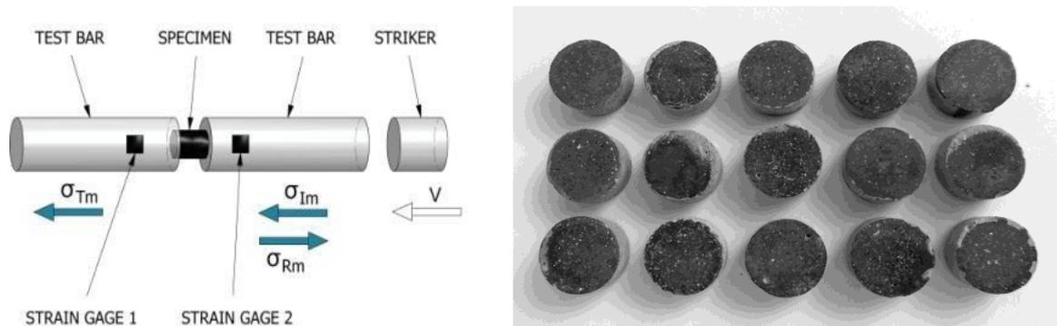
**Figure 1** Scheme of the Split Hopkinson pressure bar device (left) and specimens to be tested (right)
