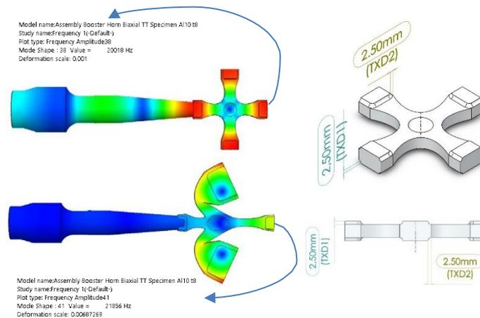
**Figure 1** – Example of results obtained from FEA after the optimization process.
