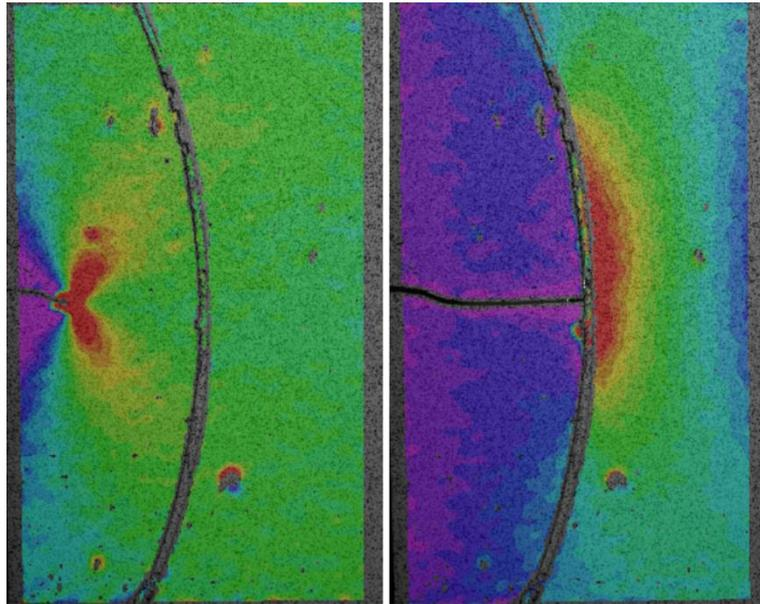
**Figure 1** - 3D digital image correlation representing vertical strain during crack propagation. The discontinuity of strain allows identifying the crack tip positions of the deflected cracks.
