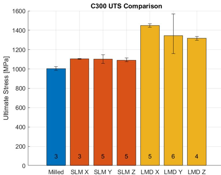
**Figure 1** – UTS comparison of C300 process and build direction
