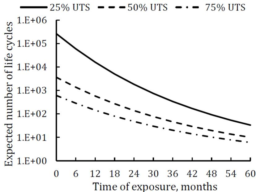
**Figure 1** – Decrease of fatigue life due to marine environment exposure
