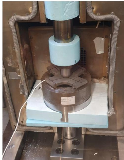
*Figure 1- Photograph of cruciform specimen experimental setup*
