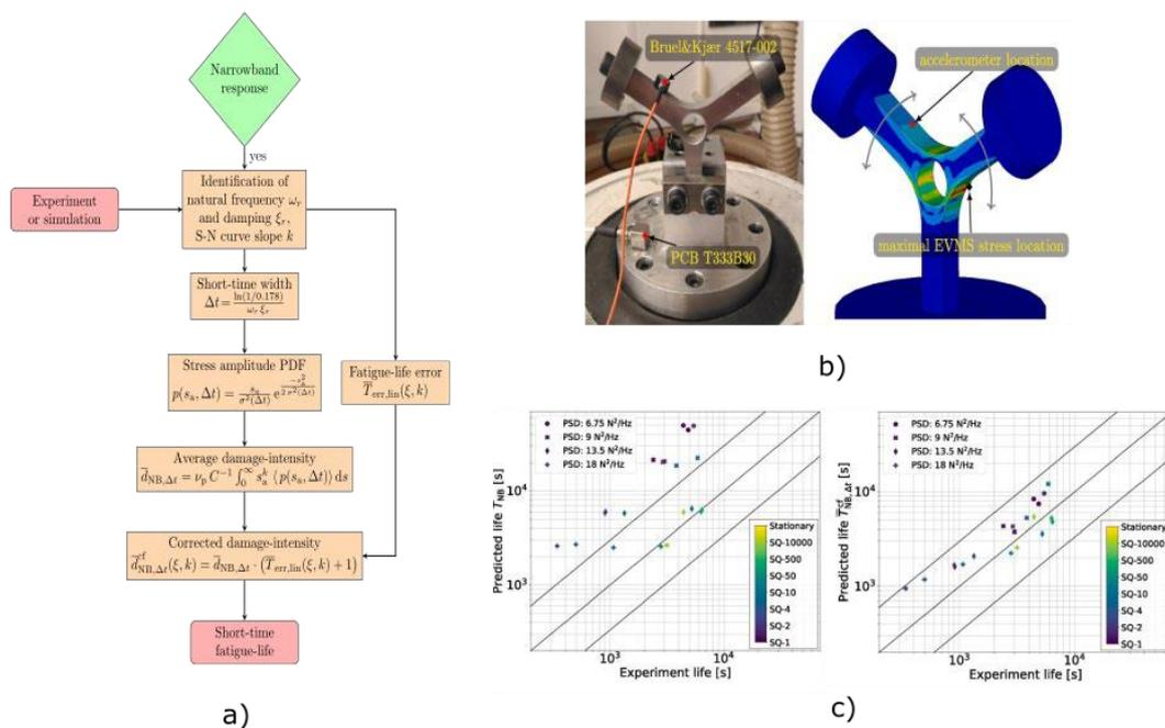
**Figure 1 - Short-time fatigue-life; a) flowchart, b) experimental setup and FEM model, c) experimental and numerically predicted fatigue life.**
