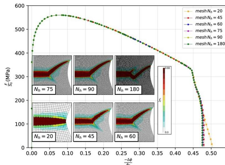
**Figure 1** – Nominal stress vs. diameter reduction for a notched round bar. Mesh size independence.
