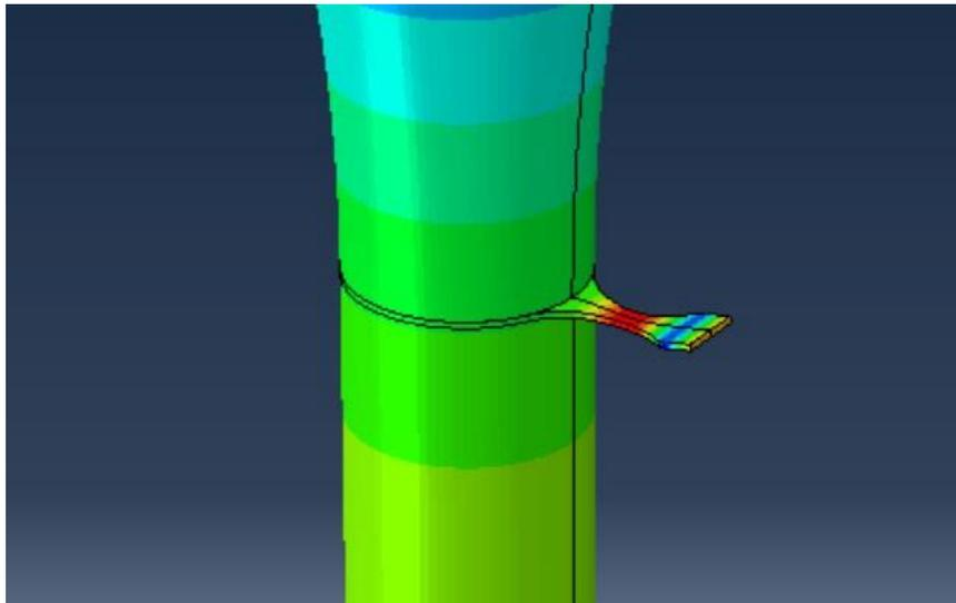
*Figure 1 – FEM 3D-model of a strip steel cantilever specimen in the ultrasonic fatigue testing system.*
