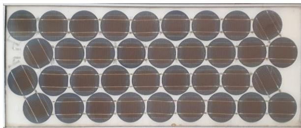
**Figure 1** - PV module installed at Auroville, India (hot and humid climate) for 14 years.
