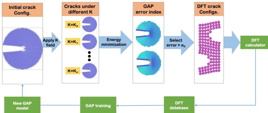
Figure 1 – Schematics of the active learning algorithm
