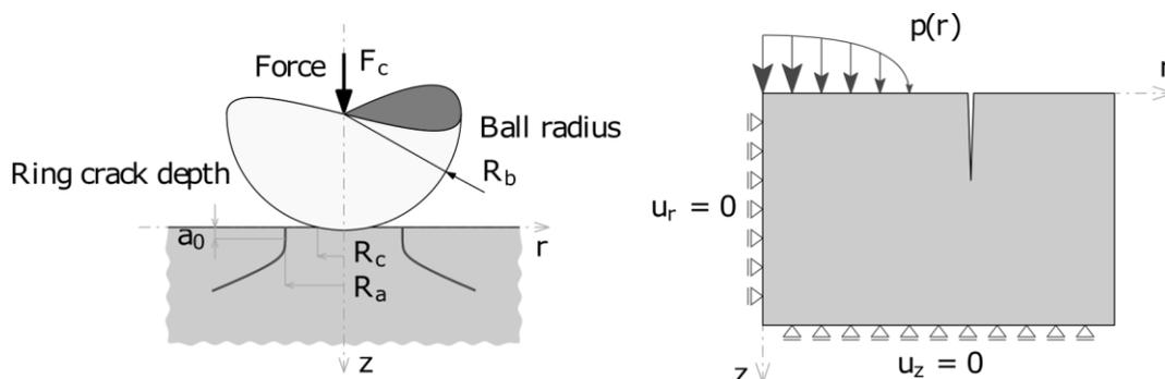
**Figure 1** – Geometry and parameters governing the crack initiation problem (left) and boundary conditions used in the computational model (right).
