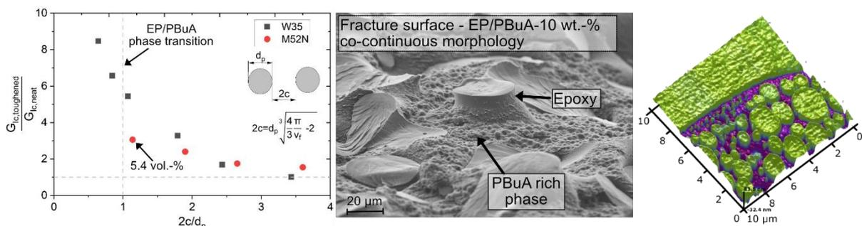
**Figure 1.** Left: Normalized critical energy release rate as a function of nanophase dimension  $d_p$  and the interparticle distance  $2c$ . Center: SEM-micrograph of the fracture surface of EP/PBuA. Right: AFM-micrograph with superposed topography and IR-spectroscopy images reveal the characteristic morphology at interphases of the composite.
