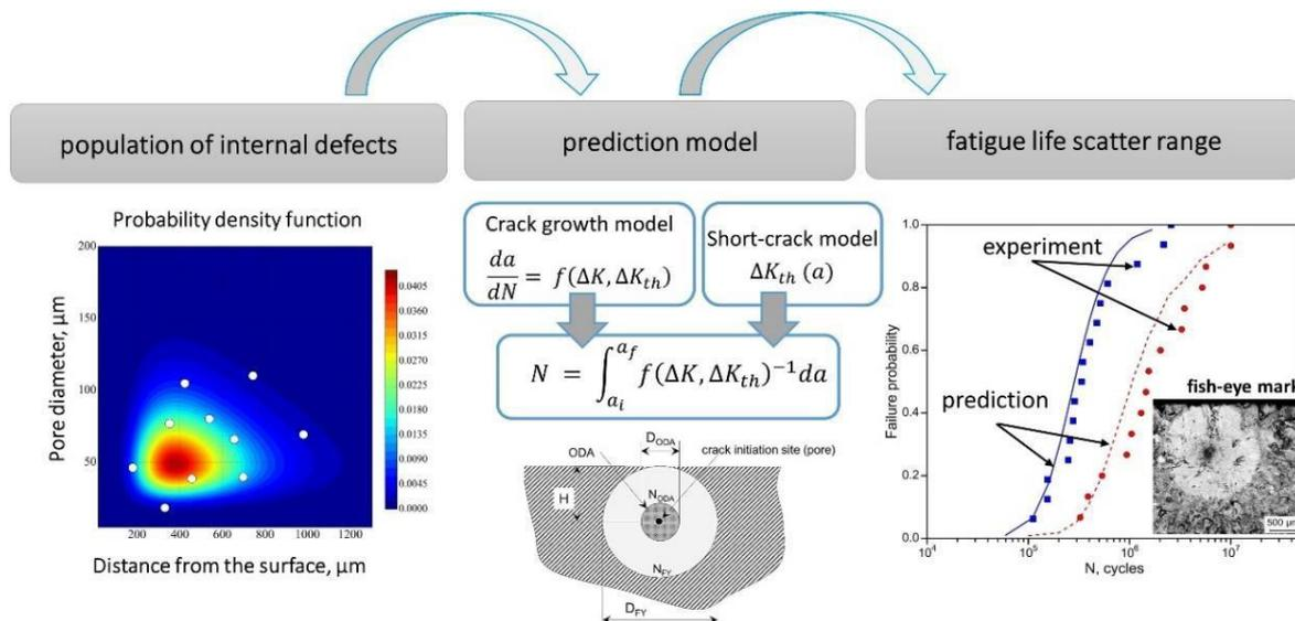
**Figure 1** - Schematic illustration of the probabilistic modelling for assessment of the lifetime scatter.
