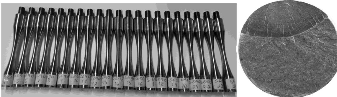
**Figure 1** – VHCF smooth specimens (right) and fracture surface of a specimen (left)
