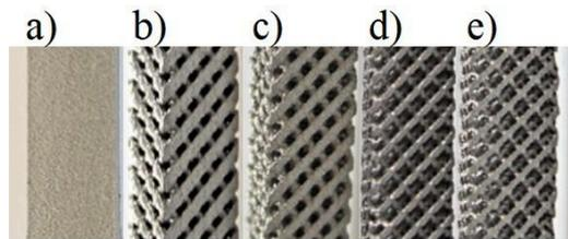
**Figure 1** - Tested additive manufactured specimens with various relative density values a) near to 1 (solid material), b) 66%, c) 50%, d) 27% and e) 18.5%.
