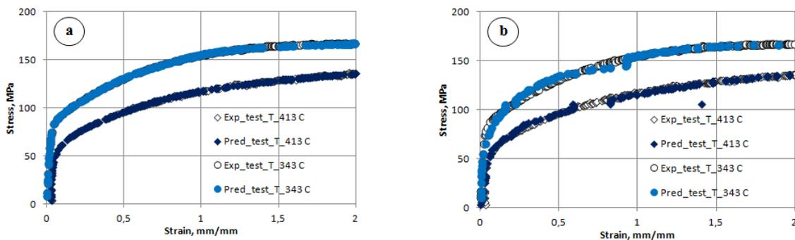
**Figure 1 - Stress-strain diagram of AL-6061 aluminum alloy at different temperatures**
