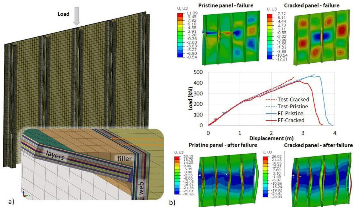
Figure 1 – a) FE model, b) Analysis results in comparison with the test
