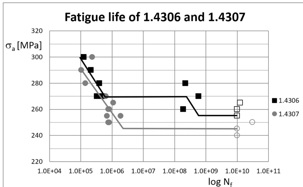
**Figure 1** – Fatigue life of studied steels. The empty points correspond to the run-out points.
