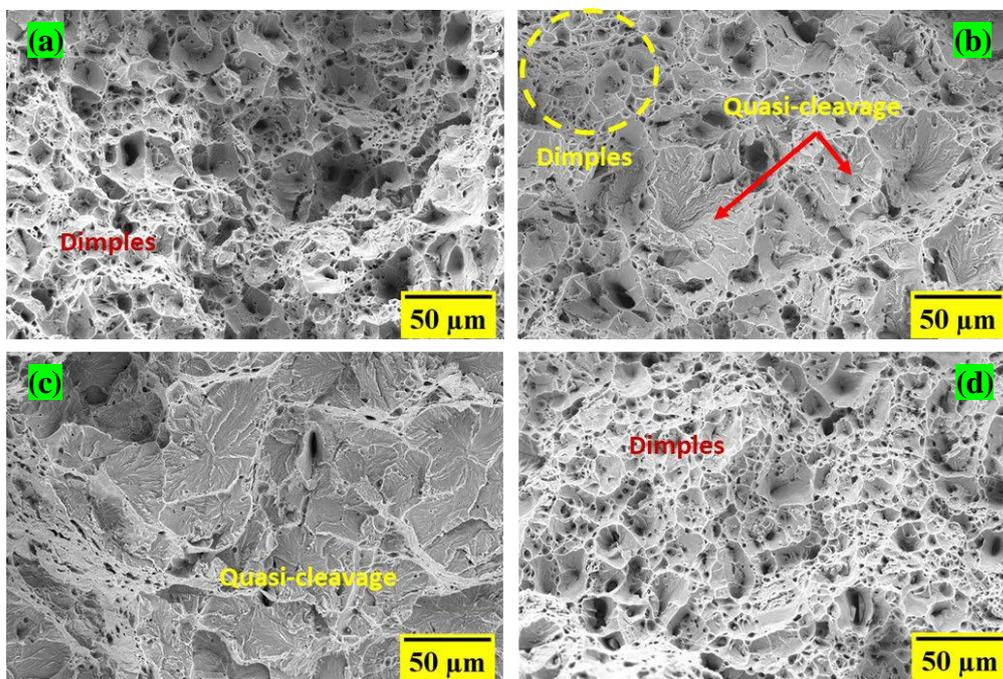
**Figure 2:** SEM images showing the fracture surfaces of (a) uncoated and uncharged (free H2), (b) uncoated and hydrogen charged for 72 hours, (c) uncoated and hydrogen charged for 90 hours, (d) coated and hydrogen charged for 90 hours.
