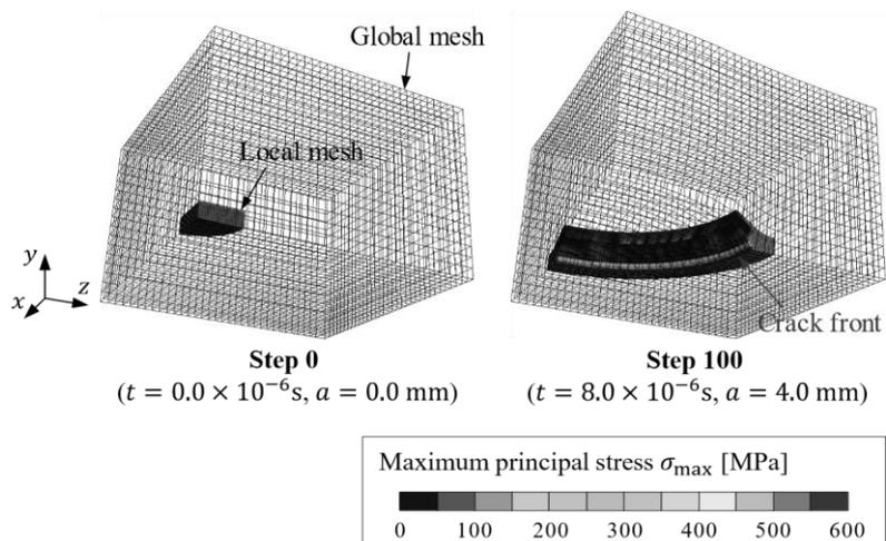
**Figure 1** – Proposed crack propagation analysis strategy example for propagating circular based on s-version FEM.
