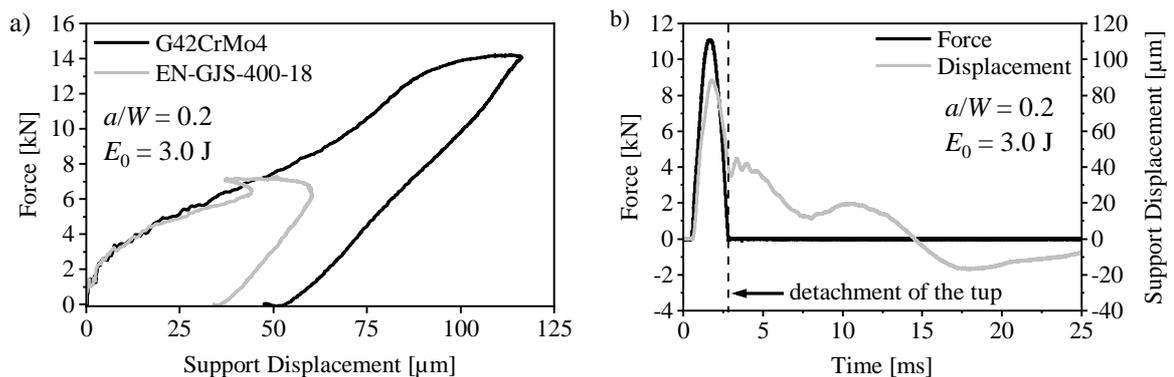
**Figure 1** – a) Force-displacement curves of the support in elastic tests for different materials, b) Force- and displacement-time curves after testing 42CrMo4
