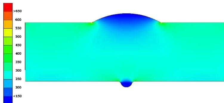
**Figure 2** FEM simulation of the V-weld of two pipes.
