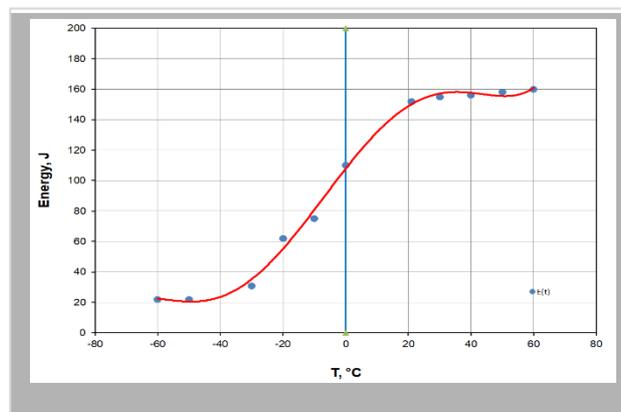
**Figure 1** – brittle to ductile transition temperature curve
