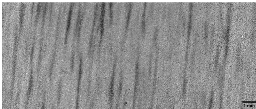
Figure 1 – overview of a segregated specimen etched using an iron chloride solution ( $\text{FeCl}_3$ ) that reveals the presence of meso-segregated regions (darker regions)
