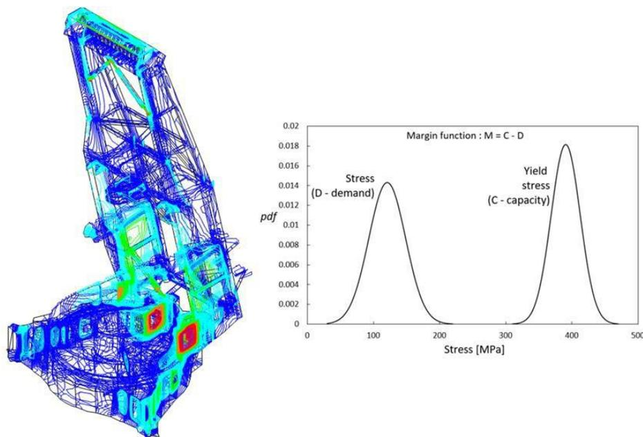
**Figure 1** – stress distribution (static load) and probability density functions, BWE.
