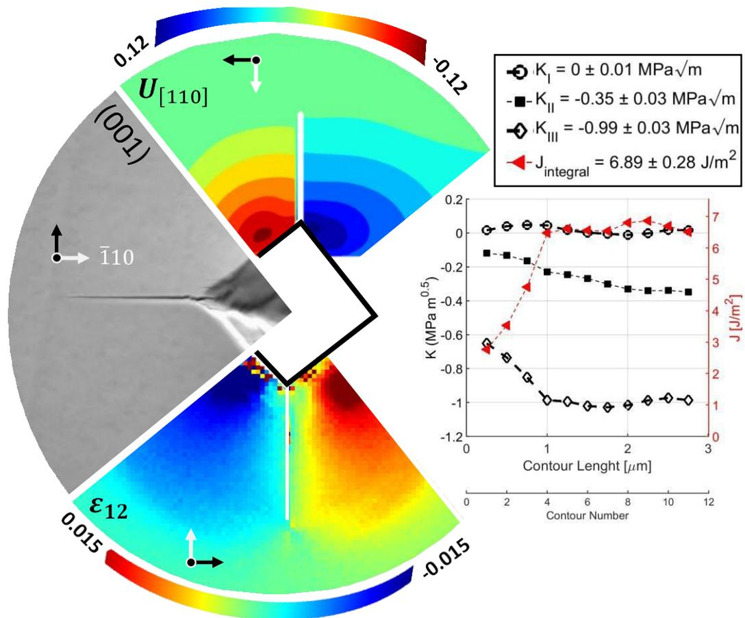
**Figure 1** – (a)  $(1\bar{1}1)$  cleavage crack due to Vickers indentation in (001) Silicon. (b) In-plane shear strain ( $\epsilon_{12}$ ). (c) Integrated displacement field in the  $[110]$  direction ( $U_y$ ). (d)  $J$ -integral and 3D SIFs (the sign of the shear modes has no physical meaning).
