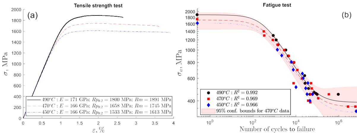
**Figure 1** – Tensile stress-strain and stress-life curves of additively manufactured MS1 maraging steel under different post heat treatments
