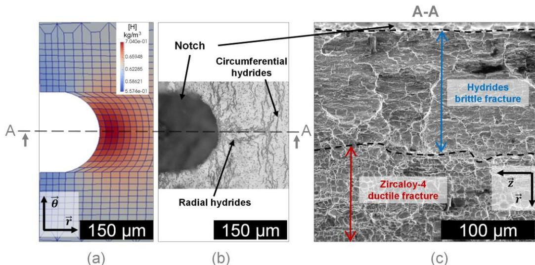
Figure 1 – (a) Finite element simulation of stress-induced diffusion of hydrogen at the initial machined notch tip; (b) Optical microscope observation of hydrides for  $KK < KK_{III}$ ; (c) MEB fractography after DHC fracture.
