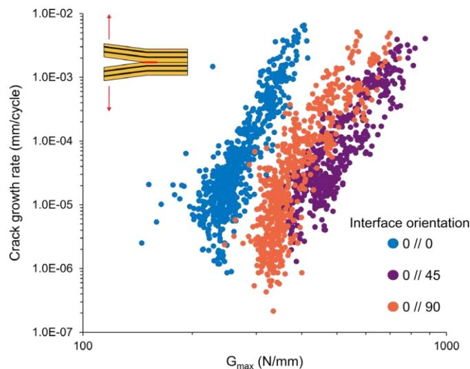
**Figure 1** – Crack growth rate curves for three of the tested interfaces. Combined results shown for 2 specimens per interface.
