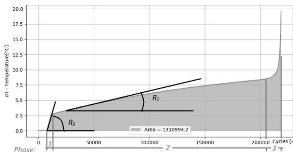
**Figure 1** – Monitored parameters of temperature evaluation during cyclic loading
