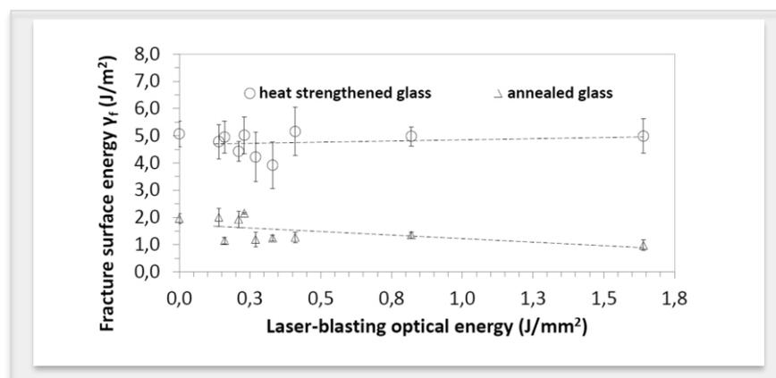
**Figure 1** – Experimental fracture surf. energy as a function of the laser-blasting energy.
