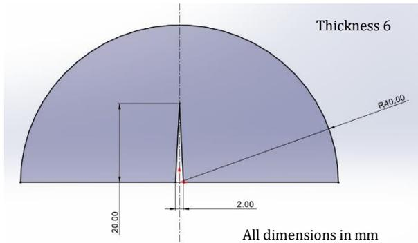
**Figure 1-** SCB specimen dimensions
