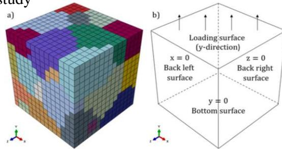
Figure 1 - a) The RVE containing 41 grains, created using DREAM.3D. b) The loading and boundary conditions applied to the RVE
