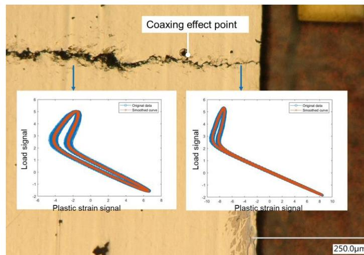
**Figure 1** – plastic strain energy variation by compliance method
