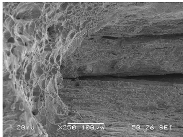
**Figure 1** – Failed surface of a plain tensile test with in situ hydrogen charging. Ductile versus brittle micromechanisms
