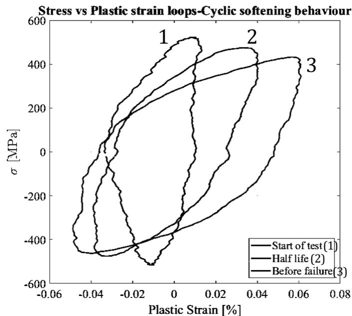
Figure 1 – Plastic strain evolution during fatigue testing
