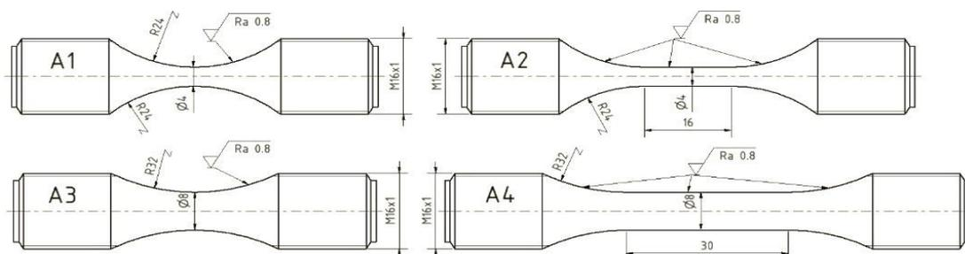
**Figure 1** – unnotched specimens used in the experiments
