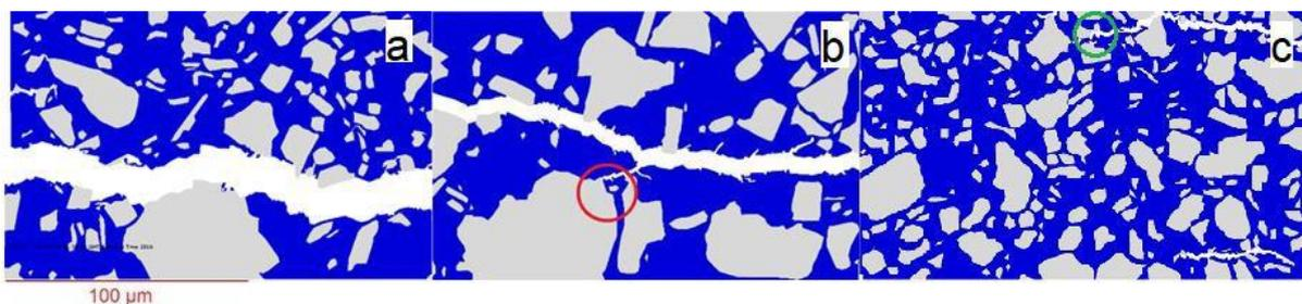
**Figure 1** Typical crack growth path (a) without arrest nor agglomeration-induced matrix crack, (b) with arrest, marked by the red circle and (c) with agglomeration-induced matrix crack, marked by green circle.
