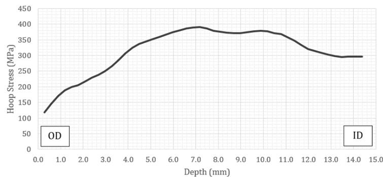
Figure 1- Contour plot showing averaged hoop stress through thickness of the weldment, OD is outer diameter and ID is inner diameter
