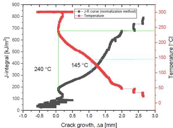
**Figure 1** - Comparison of the temperature and the effect on the shape of the J-R curve, for specimen 5.3.
