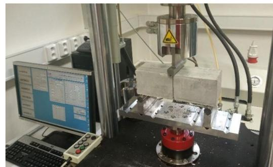
**Figure 1** – Sketch of a fatigue specimen and experimental set up for fatigue measurement.
