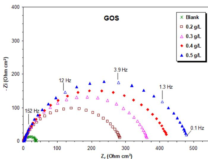
Figure 1. Nyquist plots of the corrosion of carbon steel with different concentrations of GOS at 298 K.
