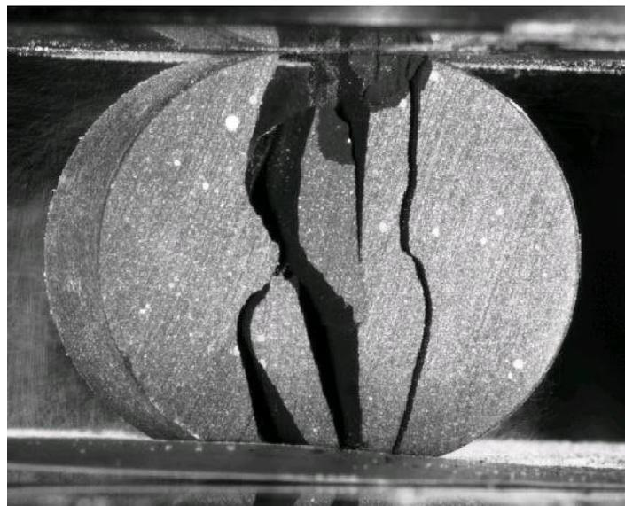
*Figure 1 - View of a BDT specimen after failure*
