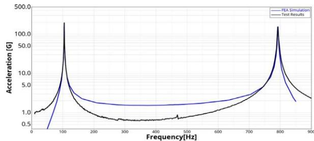
**Figure 2** – Frequency Response Functions: Experimental test vs. numerical model
