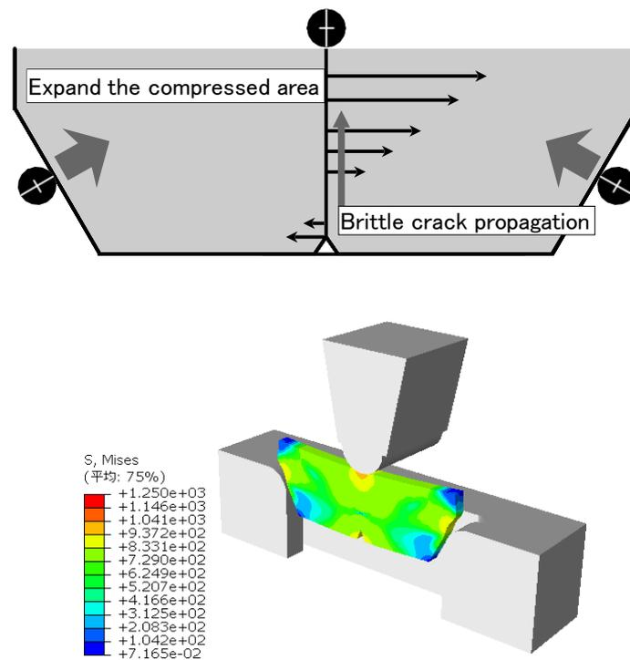
*Figure 1 – outline of newly proposed compact arrest test*
