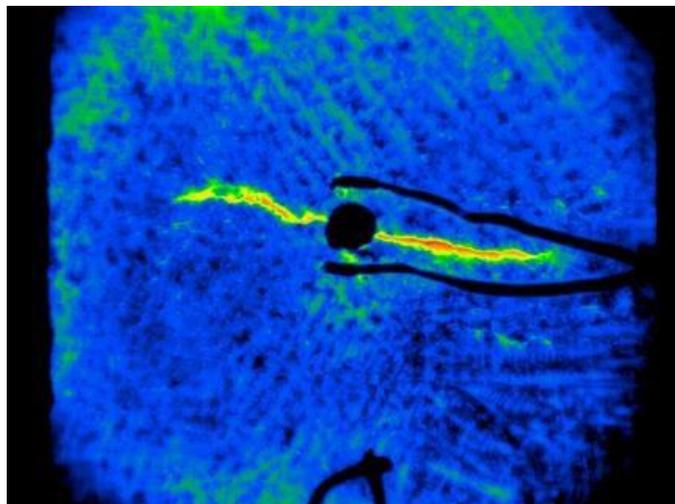
**Figure 1** – Cracks emanating from a cylindrical hole in a flat LCF specimen
