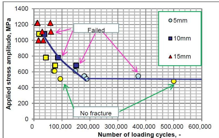
Figure 2 – Results of combined fatigue loading
