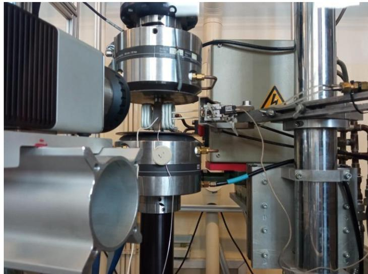
**Figure 1** – *Experimental setup for crack propagation experiments*
