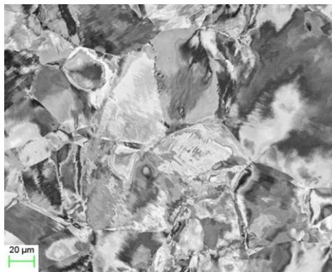
Fig. 1 Strain localization and grain fragmentation
