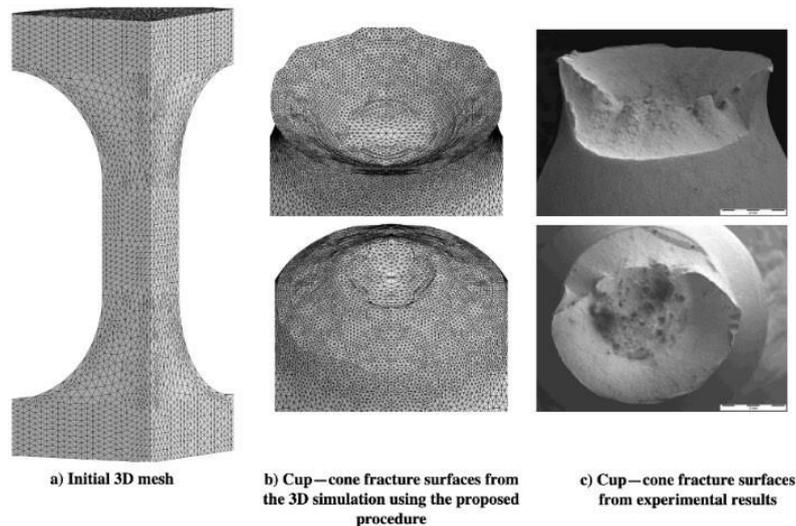
**Figure 1** –predicted cup–cone crack surfaces are smooth, well defined, and qualitatively in agreement with what can be expected from the experimental results
