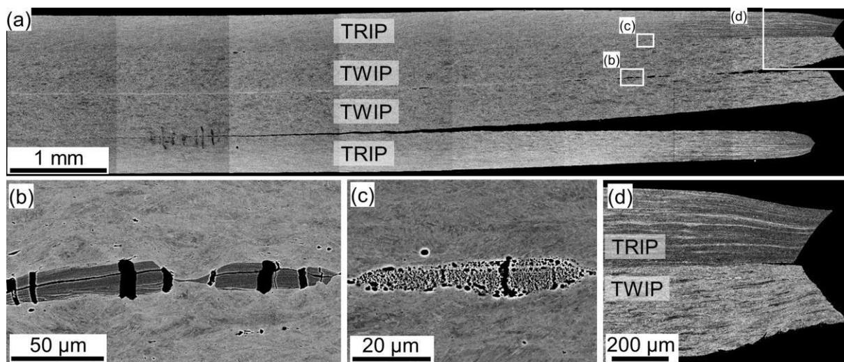
**Figure 1** - Back scattered electron (BSE) images of a tensile specimen cross-sectioned parallel to the loading axis after failure. (a) Overall view with the indication of layers. Magnified views of the (b) annealed deformation lens, (c) non-annealed deformation lenses, (d) fully bonded TRIP/TWIP interface.
