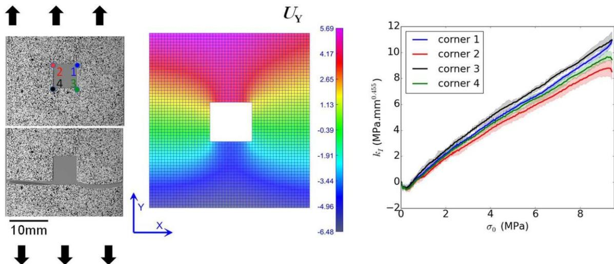
**Figure 1** – Description of the methodology, (left) tensile test with a speckle to (center) DIC for extracting the displacement field and (right) derived the generalized stress intensity factor.
