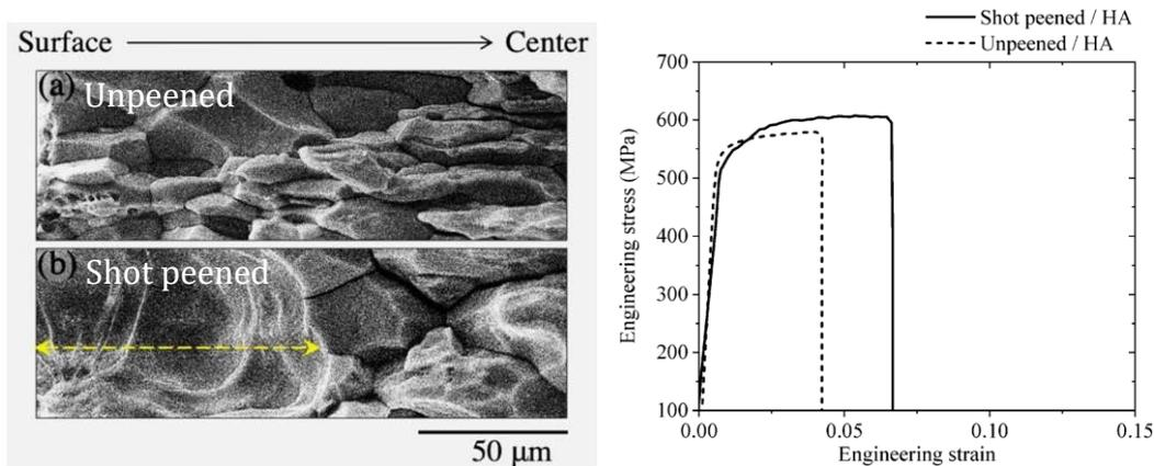
**Figure 1** – An example of processing route effects on the microstructure and hydrogen embrittlement behavior of aluminum alloys.
