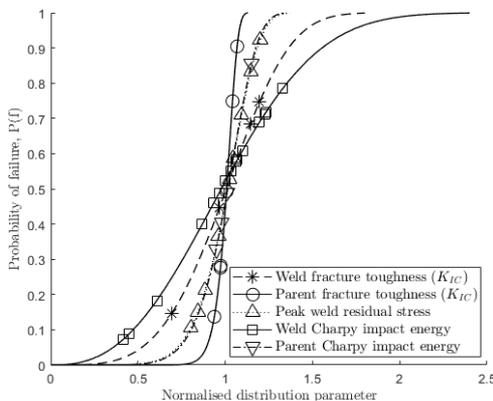
Figure 1 - Normalised Weibull CDF probability of failure vs. applied distribution parameter distributions derived from the experimental parent and weld fracture toughness ( $K_{IC}$ ), parent and weld Charpy impact energy and peak welding
