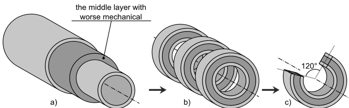
**Figure 1** – Scheme of procedure of creating axially slit rings.
