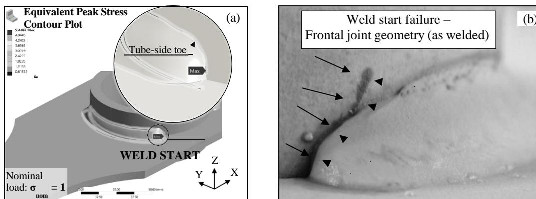
**Figure 1** – (a) Fatigue assessment of the frontal joints with the 3D scanned geometry of the weld ends according to the PSM. (b) Example of failure analysis of the frontal joints.
