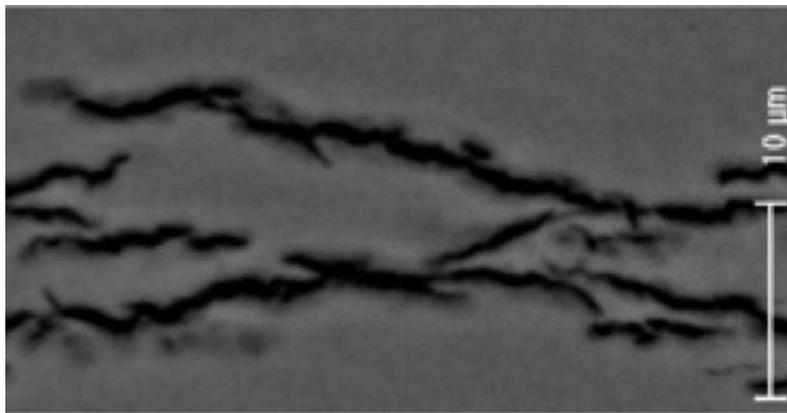
*Figure 1 - Typical cluster of zirconium hydride platelets*
