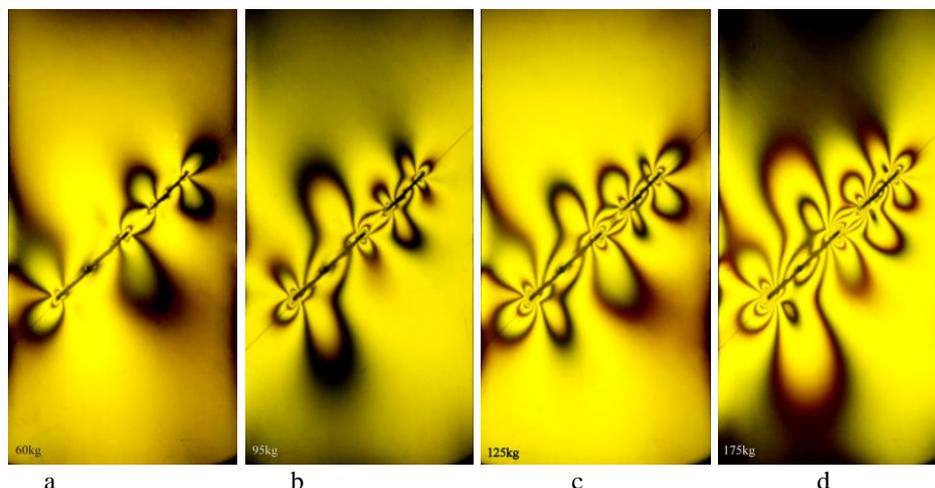
**Figure 1** - Experimental specimens tested: isochromatic fringe pattern of the plate with two collinear cracks under different loads (a-d)
