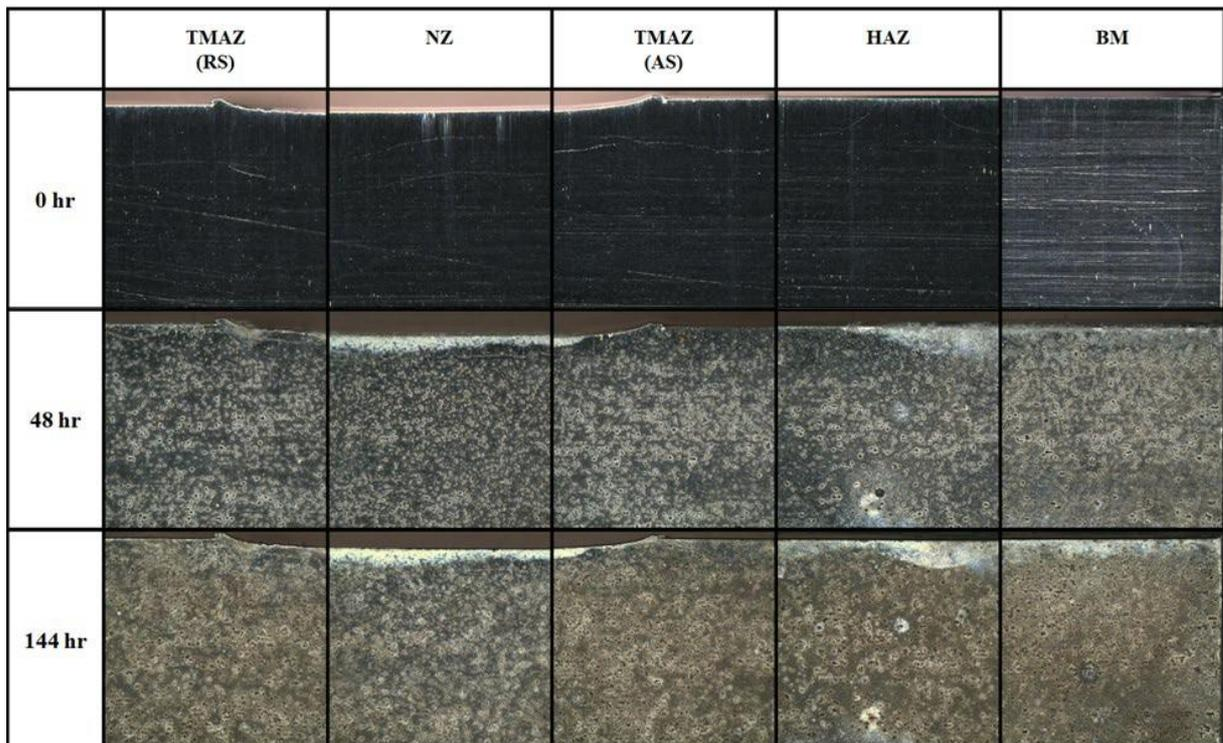
*Figure 1 Appearance in NaCl solution*
