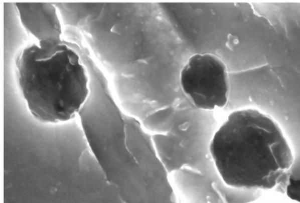
**Figure 1 – Fish eye at HE fracture**
