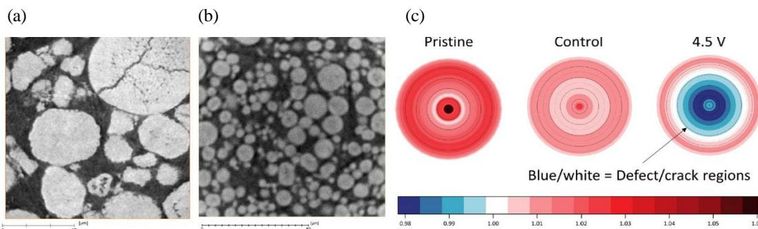
Figure 1 (a) high resolution CT slice, (b) low resolution 3D volume (c) identification of particle defects from low resolution CT scans and accompanying algorithm
