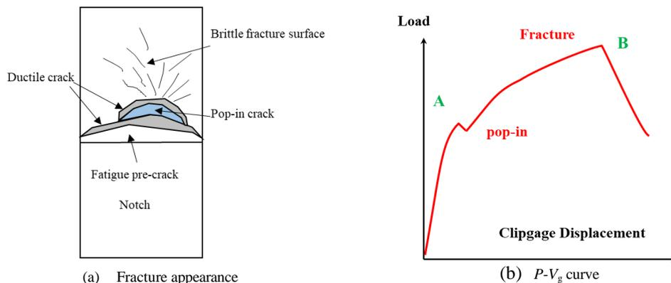
**Figure 1** – Typical pop-in which is sometimes seen in CTOD test of steel weldments
