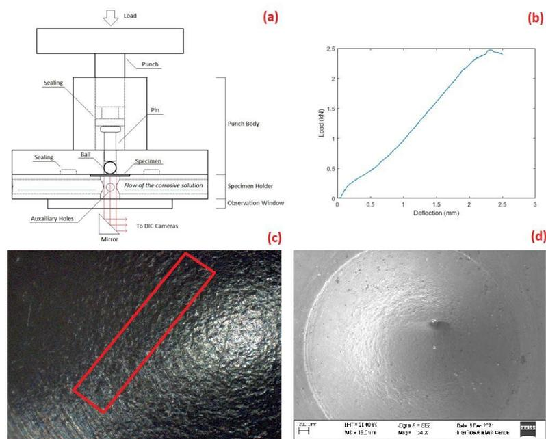
Figure 1 – (a) corrosion SPT setup; (b) load and displacement curve of a SPT sample; (c) optical microscope image and (d) SEM image of the preliminary test sample
