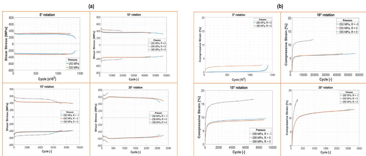
**Figure 1** - (a) Plots of shear stresses against cycles to failure for 5 degrees, 10 degrees, 15 degrees and 20 degrees angle range and (b) Plots of axial strains against cycles to failure for 5 degrees, 10 degrees, 15 degrees and 20 degrees angle range.
