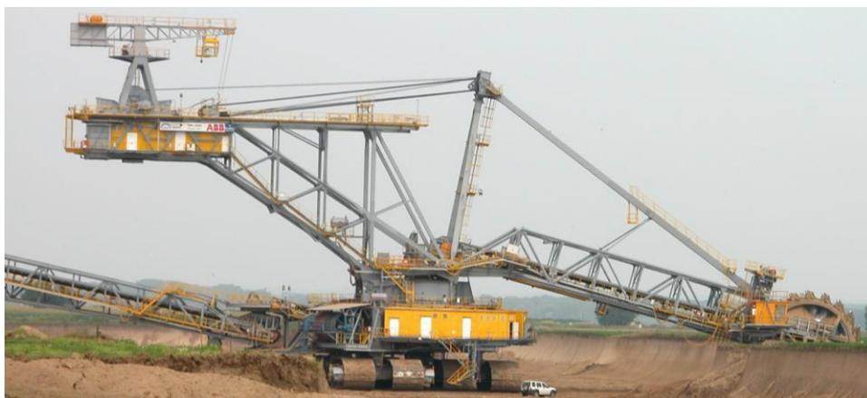
**Figure 1** - The bucket wheel excavator SRs 2000 20/5 in exploitation, Kostolac (Serbia)
