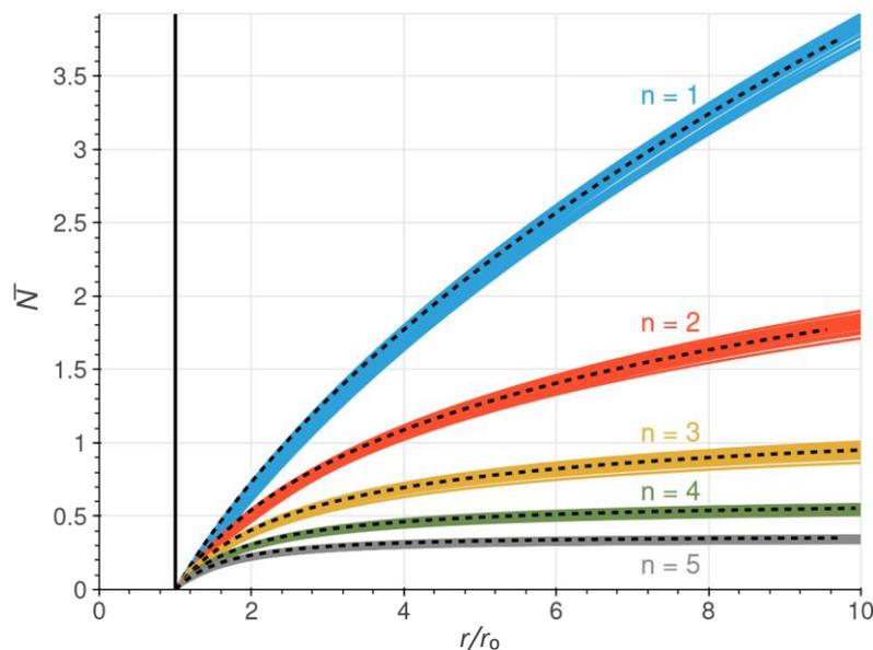
**Figure 1** – Whatever the initial crack shape the number of cycles  $N$  necessary to reach a crack of surface area  $r^2$  is the same than for a circular crack of same area.
