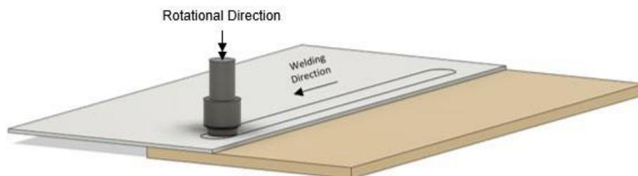
**Figure 1** – *Three-dimensional schematic of friction stir welded dissimilar aluminum to polymer matrix composite joint.*
