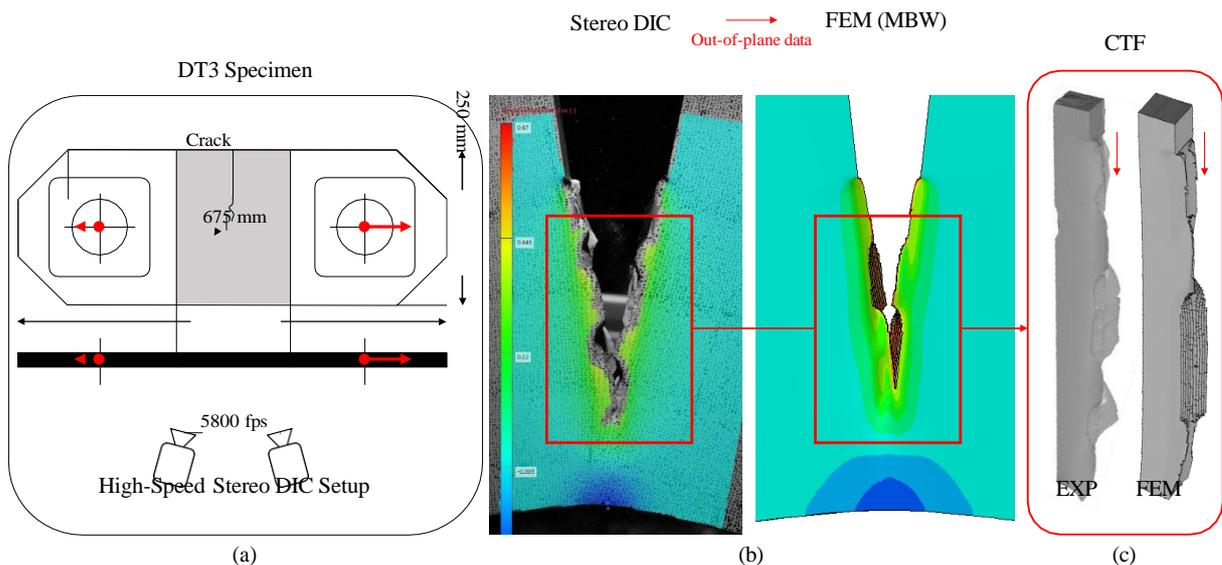
**Figure 1** - Overview of a DT3 specimen with a schematic of the High-speed Stereo DIC camera setup (a), Obtained DIC image and correlation with the numerical model (b) Experimental and numerical fracture surfaces showing Crack tip flipping phenomenon (c).
