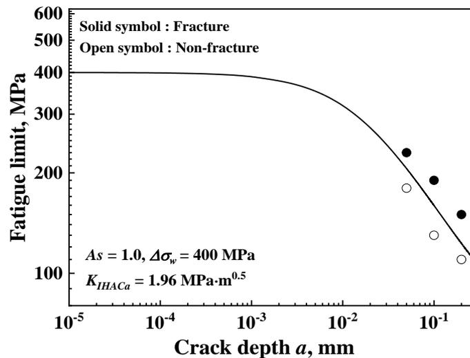
Figure 1 Relationship between fatigue limit and crack depth.
