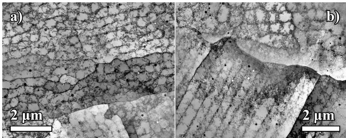
**Figure 1** - STEM micrographs (BF contrast) of the transversal foils revealing dislocation cells present prior to the testing. a) Vertical and b) horizontal building direction.
