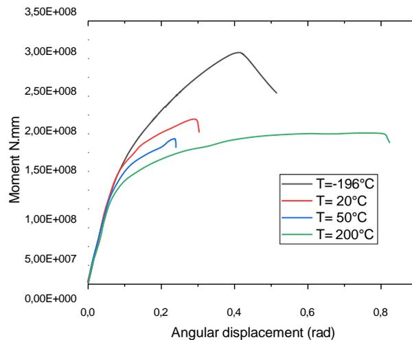
**Figure1-** End rotation vs. Moment for different temperatures degrees
