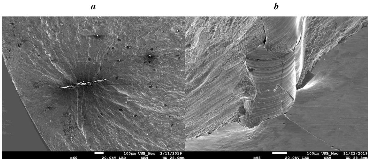
**Figure 1** – Crack initiation in non-metallic inclusion (a) and in artificial micro hole (b) seen on the fracture surface of AISI 4140 steel specimens.
