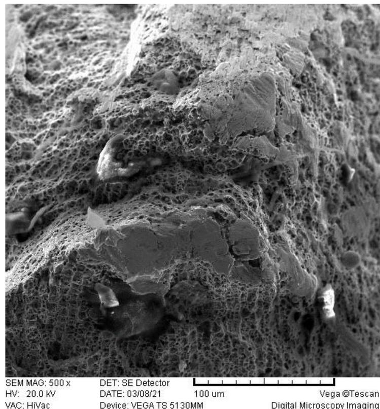
**Figure 1** – Fracture surface of the specimen C1-1
