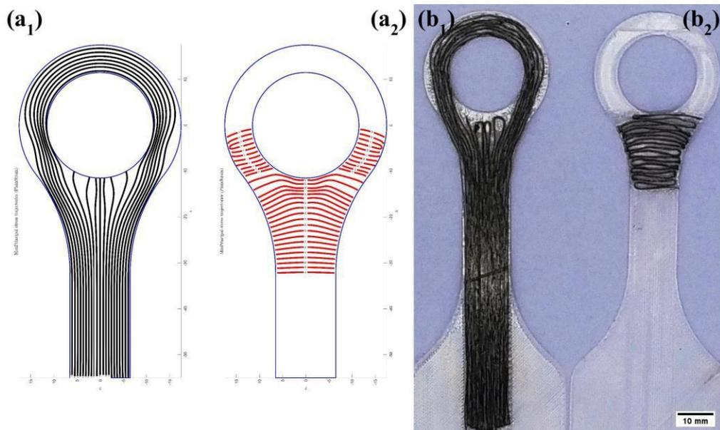
**Figure 1** Calculated fibre trajectories and photography of AM composite lugs using research oriented software, (a<sub>1</sub> and a<sub>2</sub>) calculated Max. and Min. principal stress directions for fibre placement, respectively and (b<sub>1</sub> and b<sub>2</sub>) Printed single layer of lug specimen based on calculated principal stress directions.
