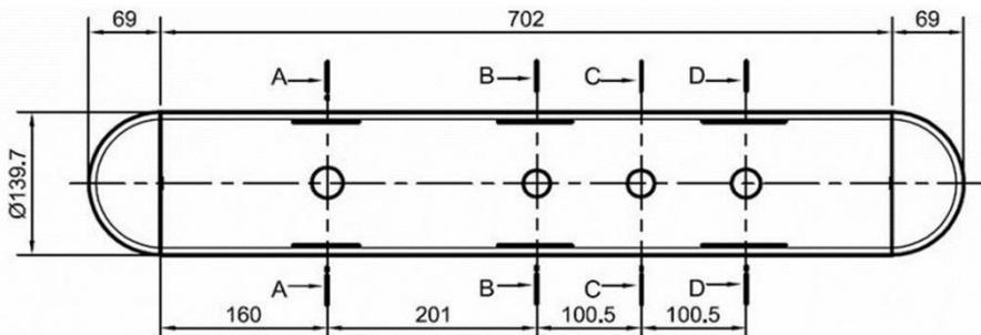
Figure 1 - Prototype with artificial defects
