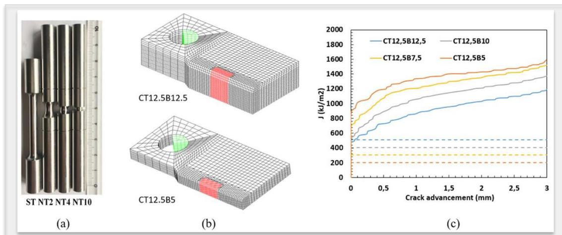
**Figure 1** – (a) Tension specimens; (b) Models de CT (c) J-R curves for CT12.5 with different thickness
