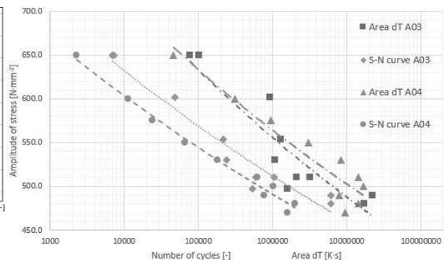
**Figure 2** – Evolution of limiting energy with S-N curves of A03 and A04 samples
