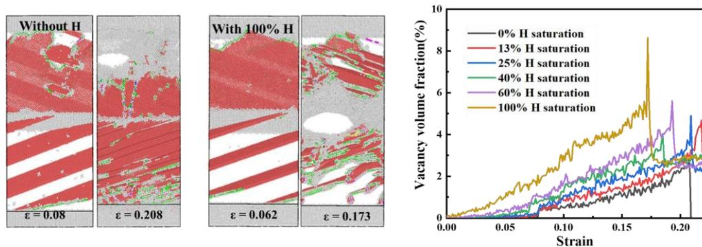
**Figure 1** – The schematic of Hydrogen-induced transgranular to intergranular fracture transition.
