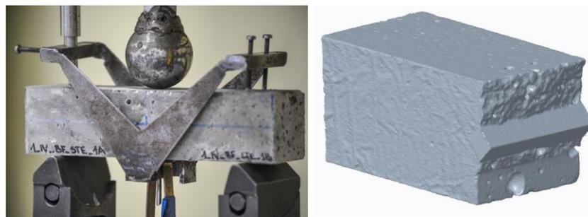
**Figure 1** – Three-point bending fracture test (on the left); specimen after fracture test.
