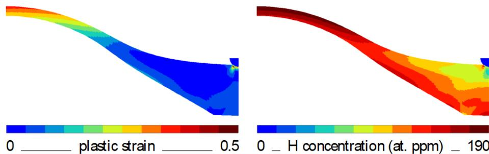
**Figure 1** – (a) Plastic strain, (b) Hydrogen concentration in the modified disk
