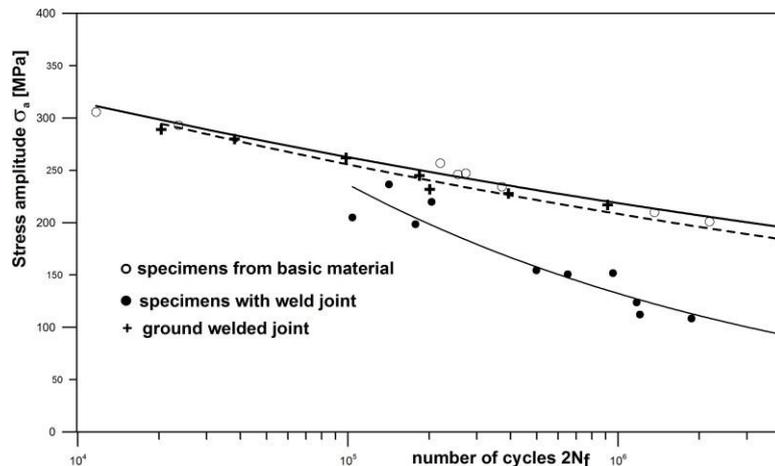
**Figure 1** Fatigue lifetime curves of those three specimen groups mentioned above (with the weld, without weld and with removed weld geometry) will be the basic for separation of the overall notch effect of the weld joint.
