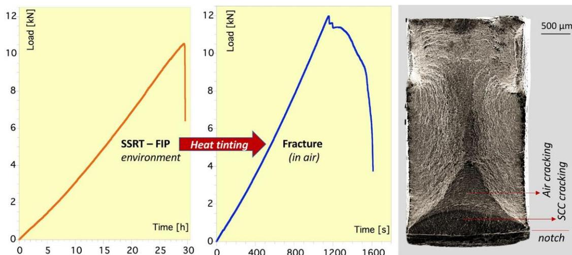
**Figure 1** – Assisted collapse of a rectangular bar specimen: a) Load – time curve in an interrupted SSRT test in FIP environment at 50°C; b) Load – time curve in subsequent tensile fracture in air; c) Front view of the fracture surface
