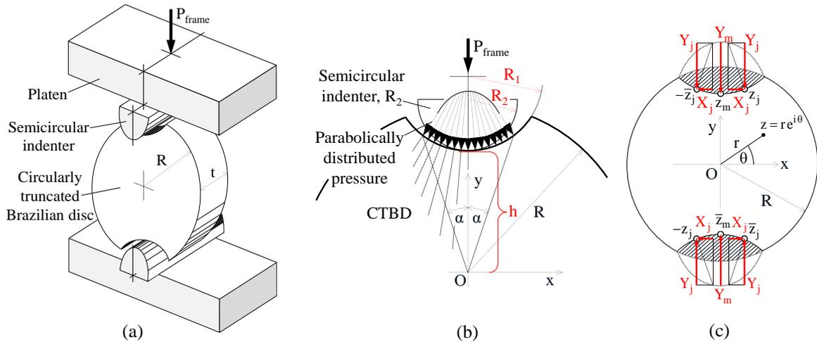
**Figure 1** - (a) The CTBD test; (b) The contact problem; (c) the 1<sup>st</sup> problem for the CTBD.
