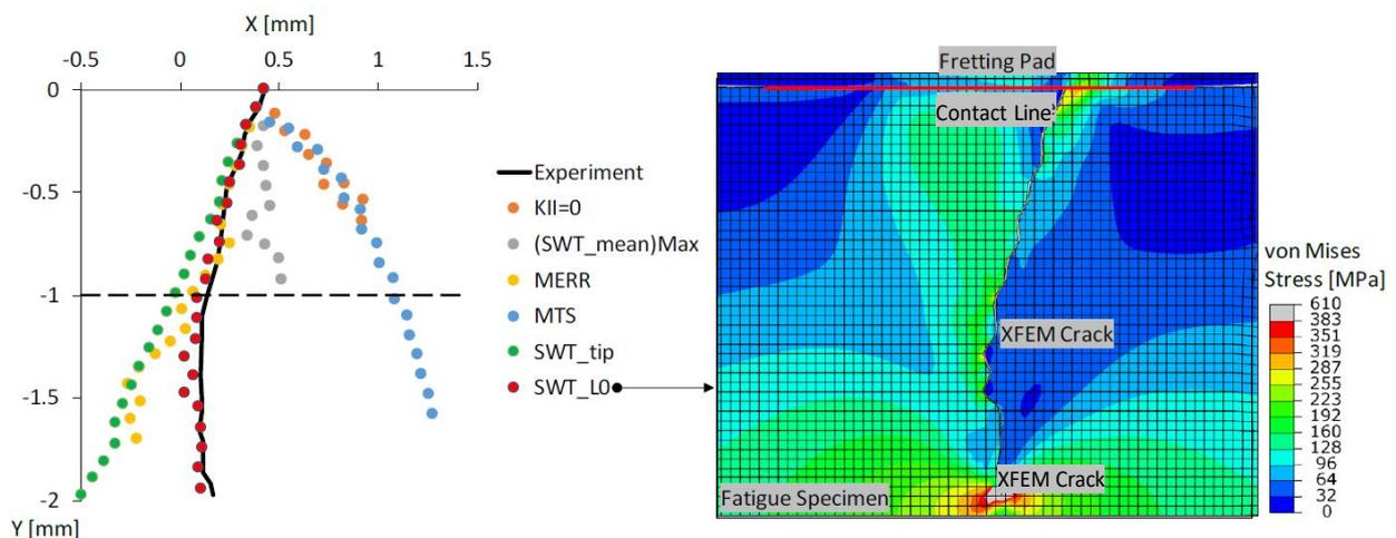
**Figure 1** – Comparing the estimated crack propagation path using different criteria and the experimental observation.
