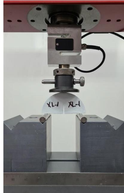
**Figure 2 –** Specimen in bending grips
