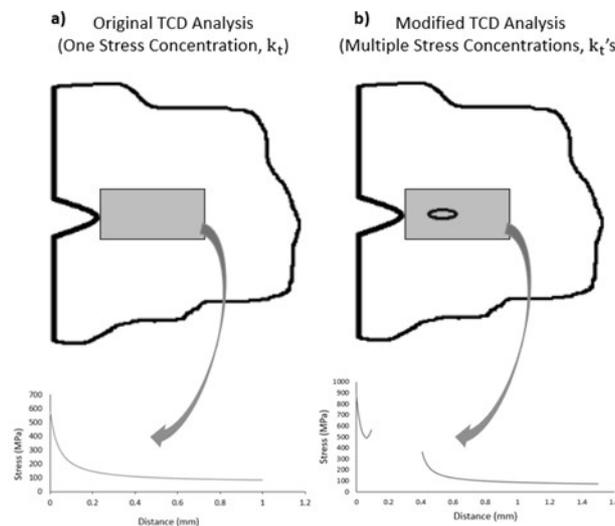
**Figure 1 - (a) Original stress-distance curve data with one stress-rising feature & (b) Interrupted stress-distance curve data due to multiple stress-rising features**
