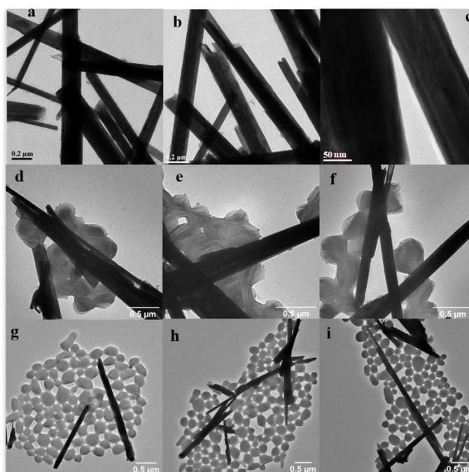
**Figure 1** - TEM images of (a–c) as prepared WS<sub>2</sub> nanotubes; (d–f) WS<sub>2</sub> nanotubes- 1.4×PTFE; (g–i) WS<sub>2</sub> nanotubes-5.6×PTFE.
