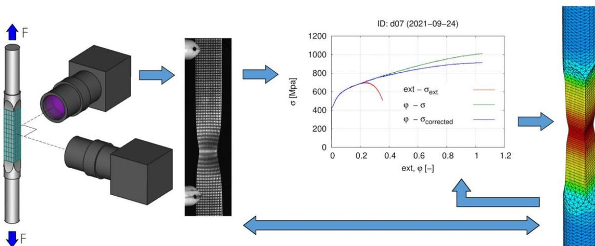
**Figure 1** – The process of obtaining the flow-curves.
