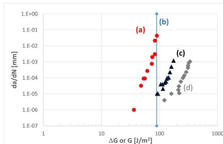
**Figure 1** –selected toughness data from literature (a) mode I fatigue fracture of neat RTM6 [3],  $\Delta K$  converted to  $\Delta G$  via an average modulus of 3000 MPa, (b) quasi-static mode I toughness of neat RTM6 [4], (c) and (d) two sets of mode I fatigue fracture of a carbon-fiber 5HS weave/RTM6 composite indicating scatter band for material and testing [5]
