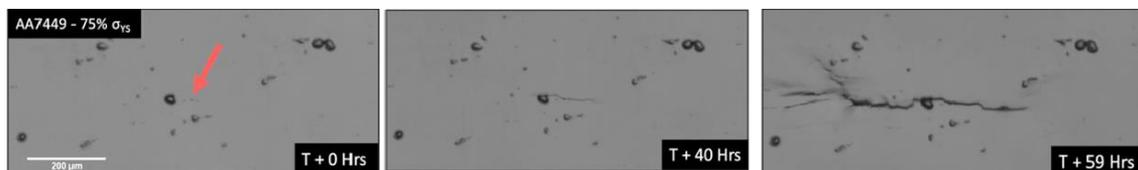
**Figure 1** – Time-lapse optical images showing the initiation of an EAC crack in AA7449 T7651 loaded to 75% of yield strength at 70 °C and 50 %RH.
