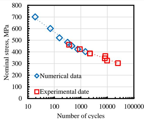
**Figure 1** - Comparison of numerical and experimental data when modeling the fatigue life of smooth cylindrical 25Cr1Mo1V steel specimens at room temperature
