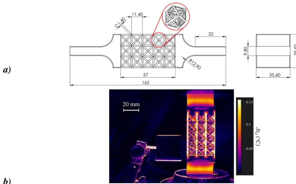
**Figure 1** – Specimen geometry used for static and fatigue testing **a)**, and total temperature variation ( $\Delta t_d$ ) after 1000 cycles at 30 Hz and 0.3 mm of displacement amplitude ( $R=-1$ ) **b)**
