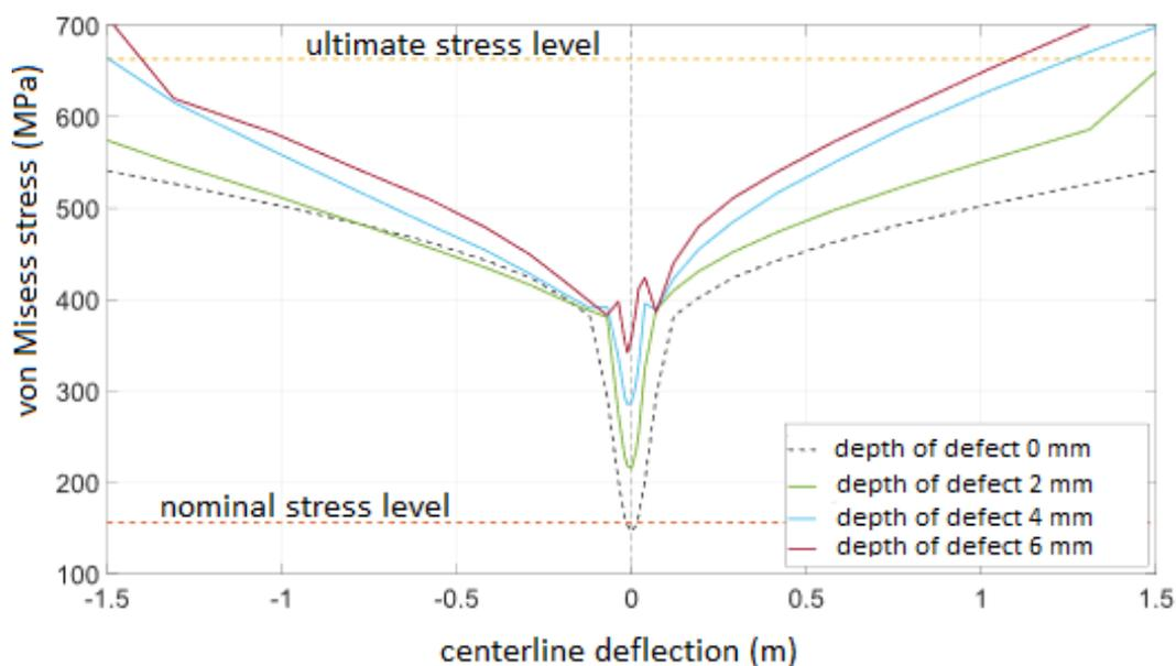
**Figure 1** Effect of additional bending (centerline deflection) on the magnitude of stresses in a corrosion defect.
