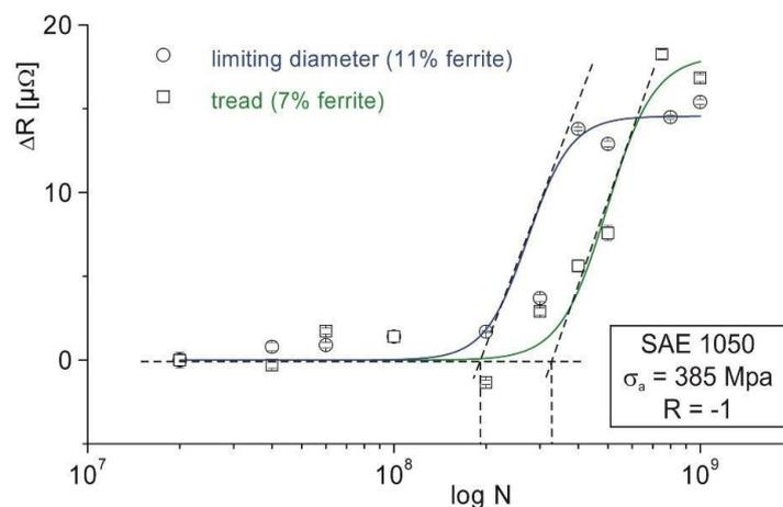
**Figure 1** - Electrical resistivity analysis of a wheel steel in the VHCF regime
