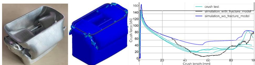
Figure 3 – WAM profile after crush test (left), Simulation of the crush test (middle), experiment vs. simulation (right)
