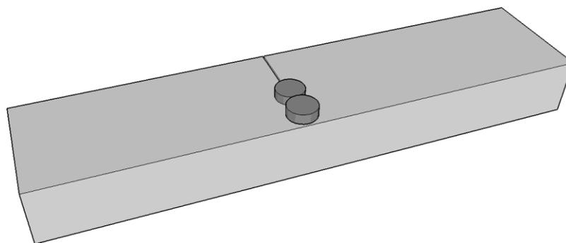
**Figure 1** – Local compression recommended in the ISO standard
