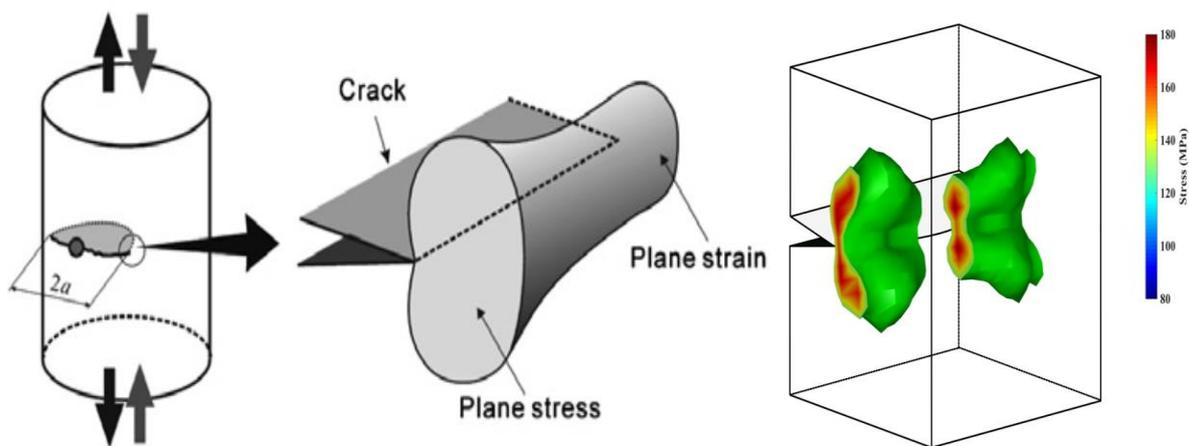
**Fig. 1:** Schematic image of plastic zone at a crack tip, in this case of a penny shape surface crack (from [1], left and middle) and iso-surface of  $\sigma_{22}$  at the 130 MPa (ratio: 1:1:30, right).
