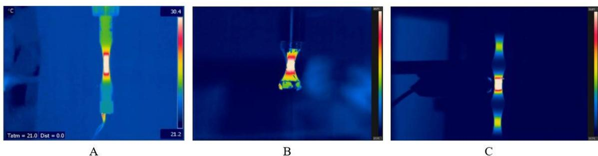
**Figure 1** – Thermographic image during ultrasonic fatigue testing in: (A) tension-compression; (B) pure torsion; (C) multiaxial Tension/Torsion
