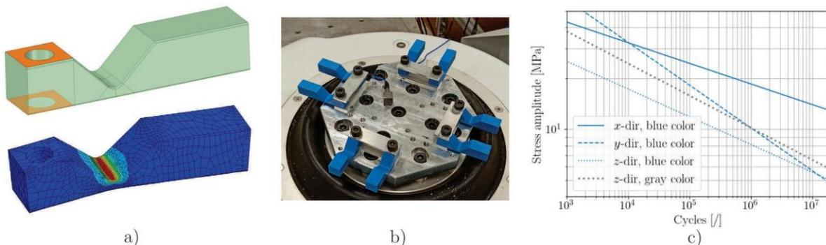
**Figure 1** – a) Specimen geometry with stress mode-shape, b) Experiment setup of 8 specimens, c) Obtained fatigue curves for tested specimen sets.
