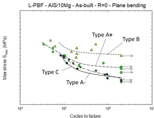
**Figure 1** – Notch fatigue behavior for  $K_t = 1.58$
