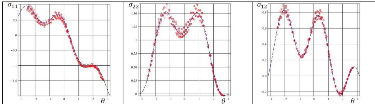
**Figure 1** - The angular distributions of stresses: atomistic solution (red points) and continuum theory (blue lines)
