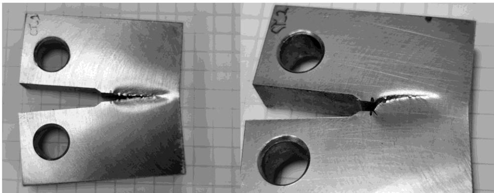
**Figure 1** – Post-rupture images of CT specimens machined with the notch parallel (left) or perpendicular (right) to the printed tracks.
