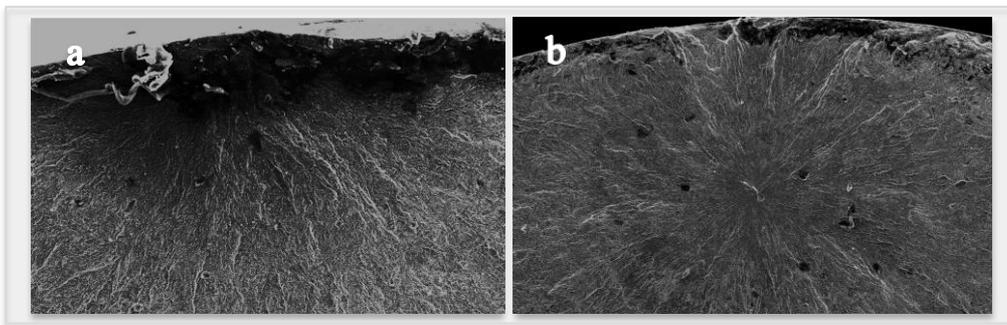
**Figure 1** – SEM images of crack initiation (a) at the surface and (b) inside the H13 specimen
