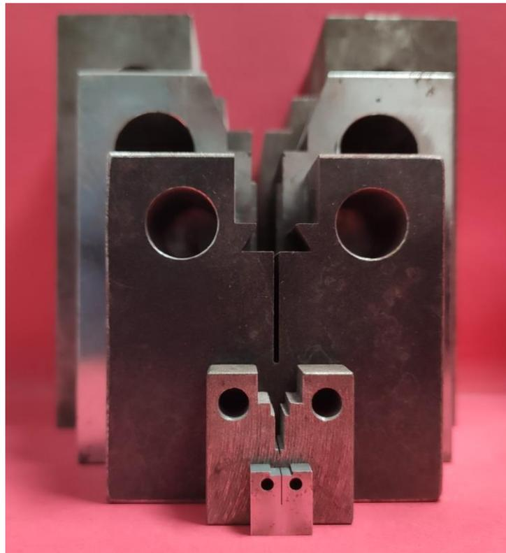
*Figure 1 – Comparison between mini-CT and standard CT specimens.*
