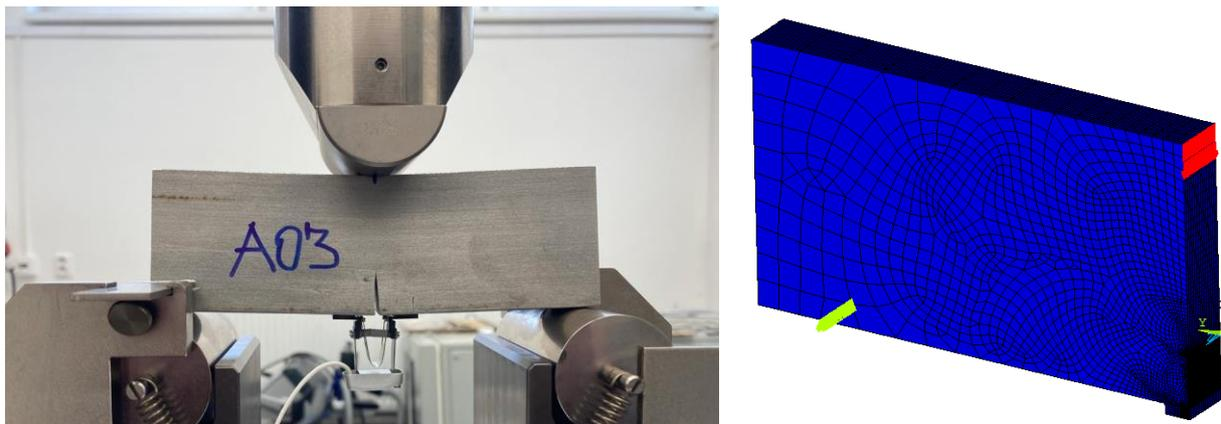
*Figure 1 – Experimental configuration and 3D model from software ANSYS.*
