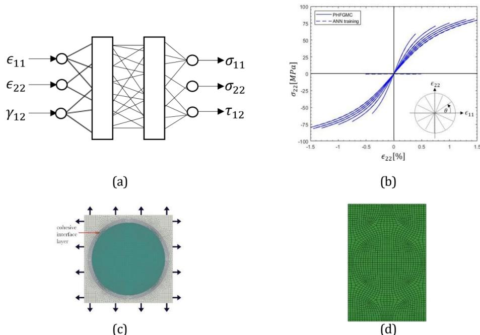
**Figure 1** – (a) Schematic representation of an ANN-micromodel where the ANN input and output include in-plane strain and stress components, respectively. (b) Prediction of a trained ANN-micromodel in the form of RUC average stress-strain responses for different strain paths. (c) A PHFGMC square RUC micromodel with interface cracks used for the ANN training data. (d) A PHFGMC hexagonal RUC micromodel with an inelastic matrix used for the ANN training data.
