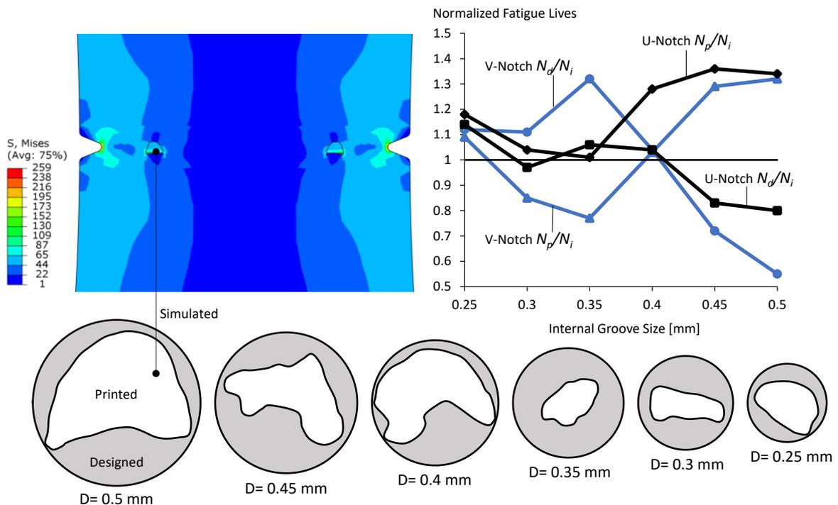
**Figure 1** – Effect of designed (d) and printed (P) internal stress relief groove on fatigue lifetime of V-Notch and U-Notch samples. The lives are normalised using lifetime of initial sample (i) without the groove
