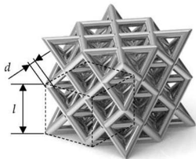
**Figure 1** – Lattice structure retained in this study with the unit cell geometry highlighted.
