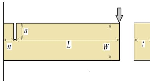
**Figure 1** - notched micro- cantilever beams.
