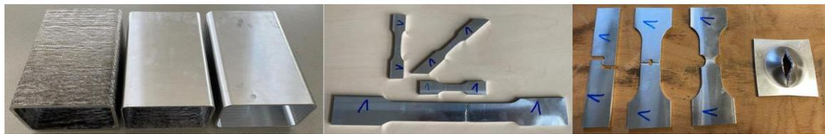
Figure 1 – WAM profiles (left), specimens for fracture characterization (middle and right)
