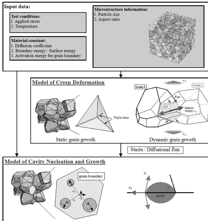
**Figure 1** - Outline of proposed integrated model for predicting deformation and cavity growth caused by Coble creep
