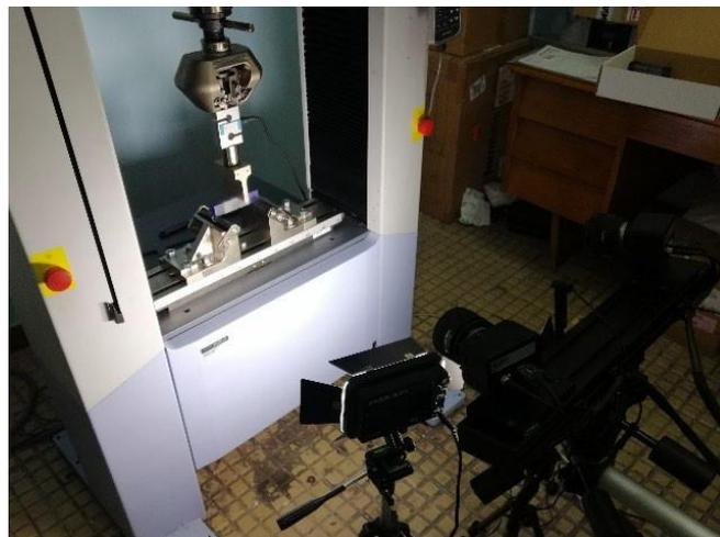
**Figure 1** – Plane-strain fracture toughness test setup with DIC dual-camera device.
