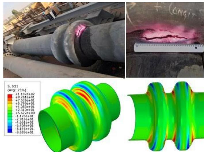
*Figure 1 -The location of circumferential crack in the expansion joint of heat exchanger.*
