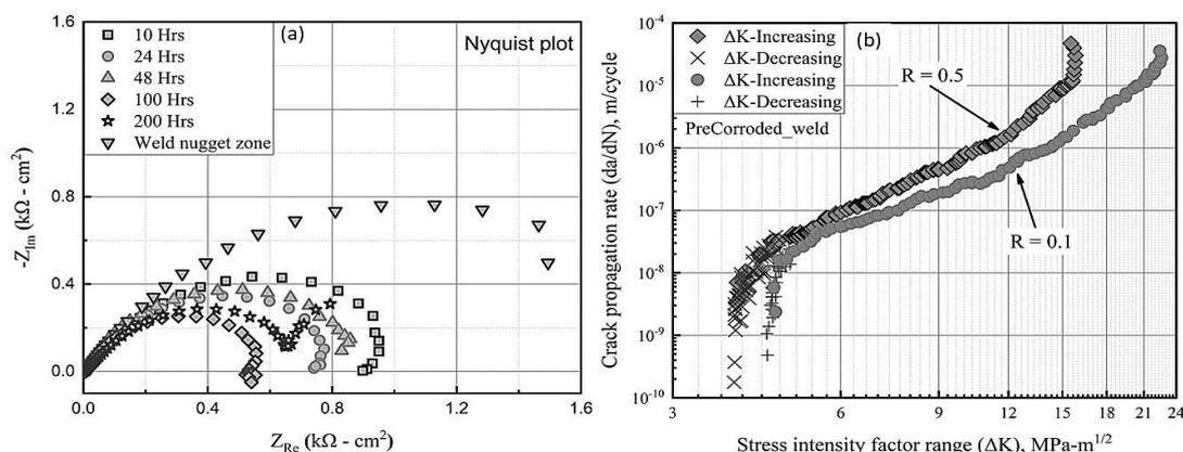
**Figure 1** – Charge transfer resistance curve (a) at different time intervals and (b) fatigue crack propagation behavior after 100 hrs. of immersion in 3.5% NaCl solution.
