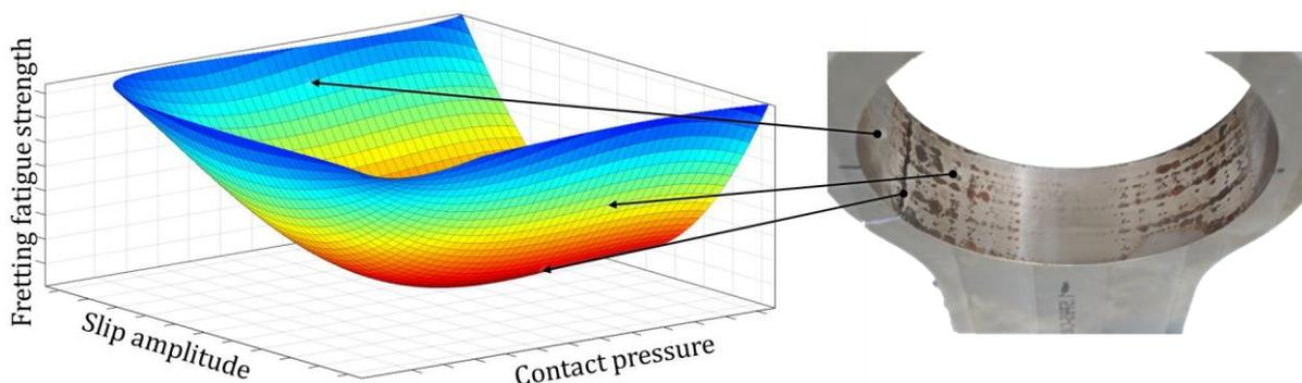
**Figure 1** - Schematic representation of the local fretting fatigue strength of a connecting rod as a function of the local parameters slip amplitude and contact pressure
