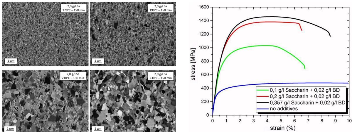
**Figure 1** – SEM images of different nc-ufg bimodal micro-structured nickel samples after different heat treatment times at the same temperature.
