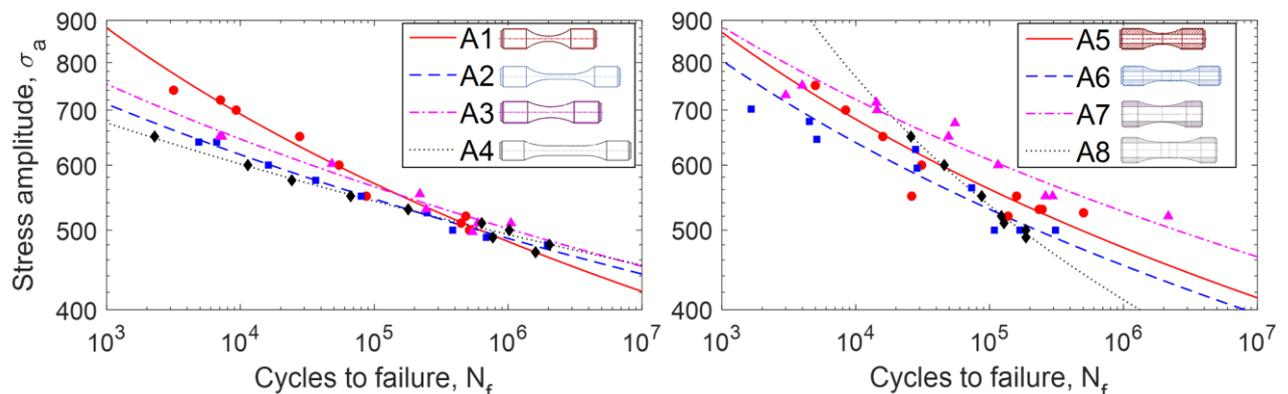
**Figure 1** – S-N model applied to data from unnotched 42CrMo4+QT steel specimens: (a) solid specimens (A1 to A4) and (b) hollow specimens (A5 to A8).
