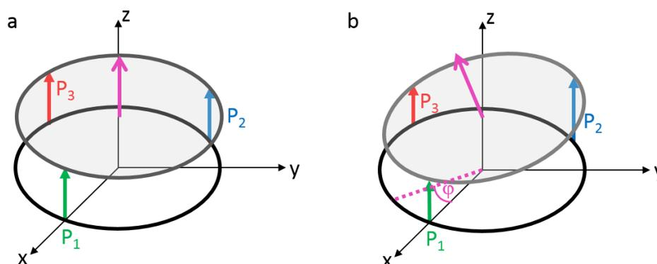
**Figure 1** – Model for determining the position of an initiated crack [1]
