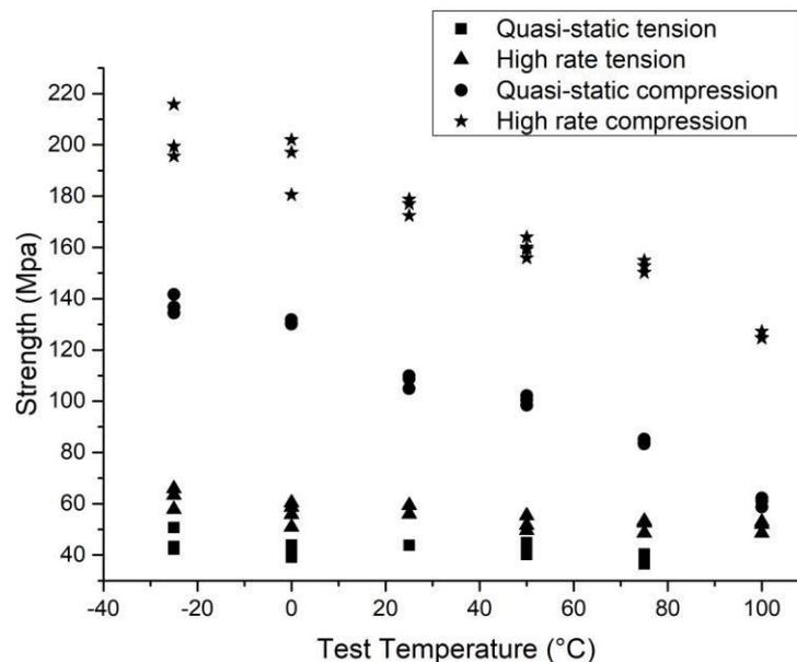
**Figure 1** - Test temperature and strain rate dependence of strength of epoxy based syntactic foam.
