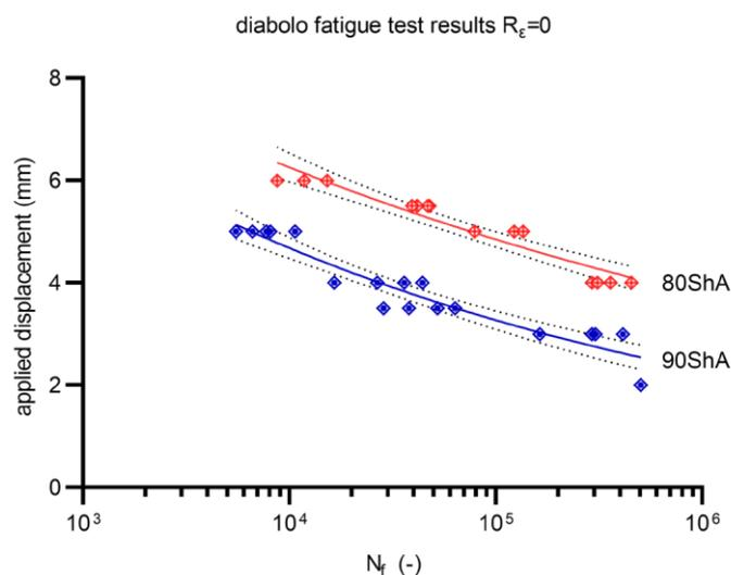
**Figure 1** – Fatigue curves for PUR elastomers (80 ShA, 90ShA) tested under displacement control mode,  $R=0$
