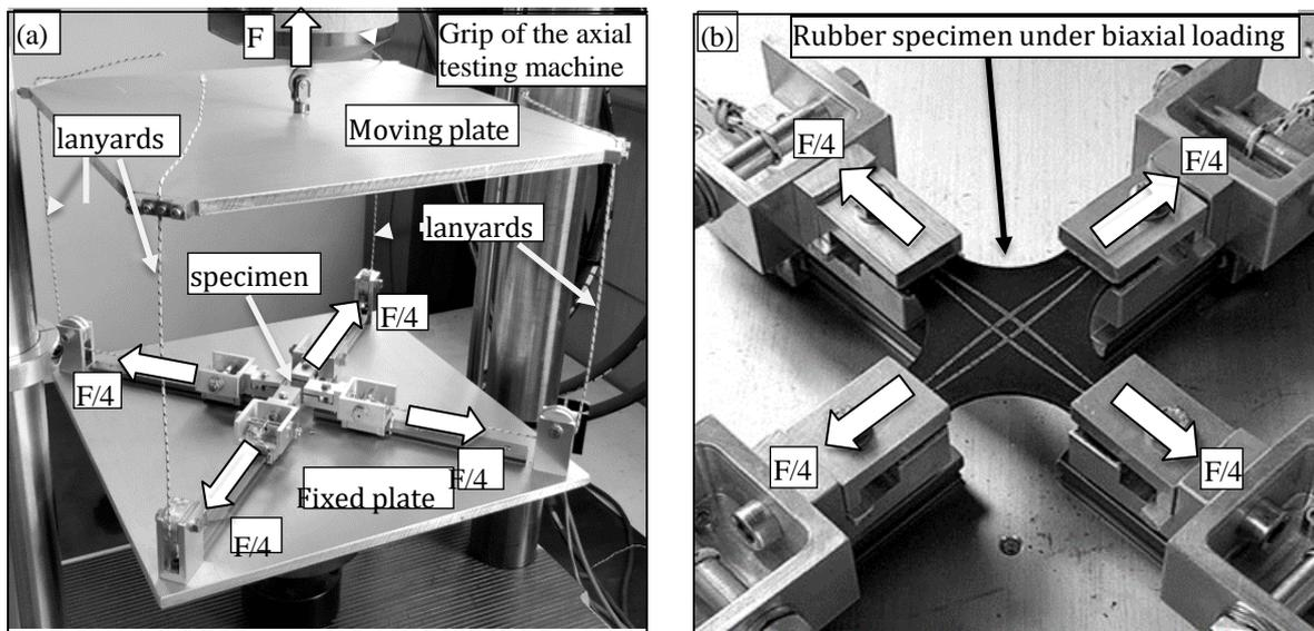
**Figure 1** – (a) Developed fixture to perform biaxial testing of rubbers using uniaxial testing machines. (b) Example of EPDM rubber cruciform specimen under biaxial loading.
