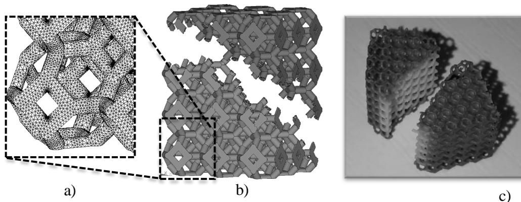
**Figure 1** – a) Detail of the FE mesh of the studied foam architecture, b) predicted fracture surface upon compressive loading, c) experimentally observed fracture.
