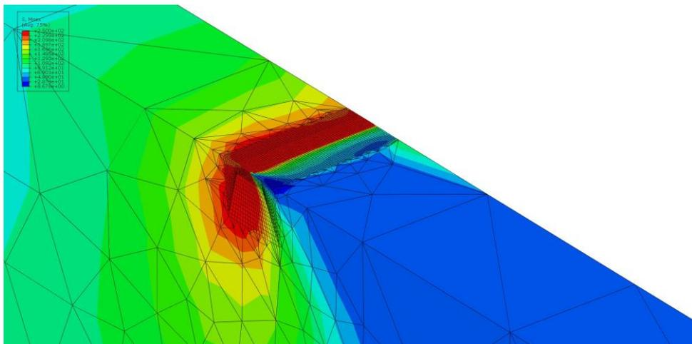
**Figure 1** – Three-dimensional model for fatigue crack growth.
