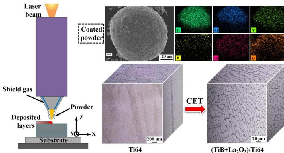
**Figure 1** – SEM of coated powder and optical microstructures of Ti64 and (5wt.% TiB<sub>2</sub>+0.5wt.% La<sub>2</sub>O<sub>3</sub>)/Ti64 fabricated by LMD
