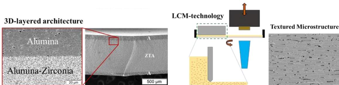
**Figure 1** – Schematic of 3D printed architectures using a multi-material approach and tailored microstructures.
