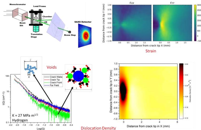
**Figure 1** – Strain, dislocation density, and a measure of pore volume near cracks grown in hydrogen (top) and air (bottom)
