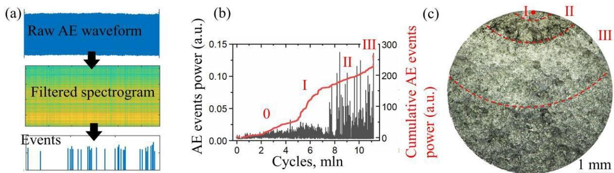
**Figure 1** – Graphical abstract of the work, showing (a) digital processing of the acoustic emission (AE) data during ultrasonic fatigue testing, (b) resulting AE activity, and (c) fracture surface a specimen after fatigue failure with fracture stages
