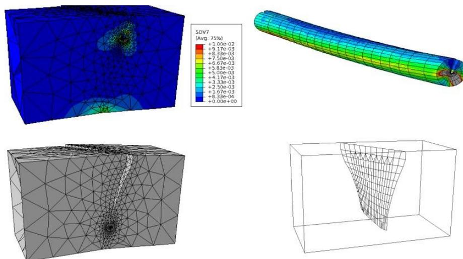
**Figure 1** – Mixed-mode crack growth in a 3PB specimen under LCF (region of crack growth is shown in the Figure); Equivalent inelastic strain in an intermediate crack growth step, the focused mesh around the crack showing the opening; Mesh details of the final crack shape; Final crack surface after the simulation.
