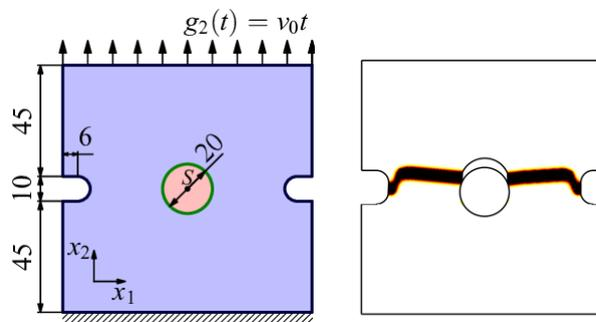
**Figure 1** – interface and bulk cracks.
