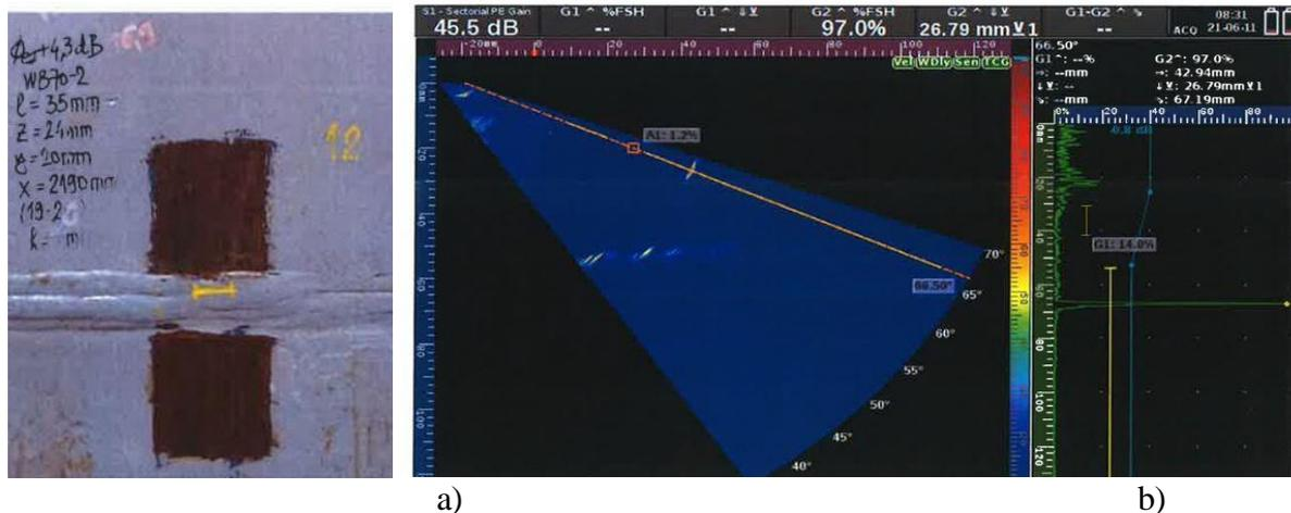
Figure 1 – UT indications: a) marked on the outer surface, b) as seen on the screen.
