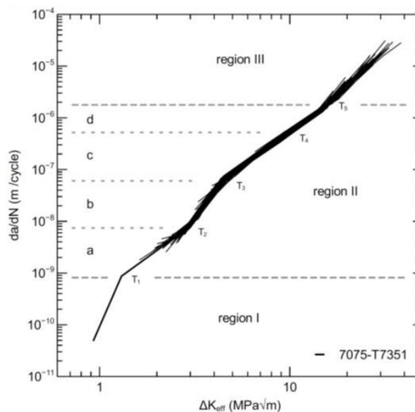
**Figure 1** - FCGR master curve as a function of  $\Delta K_{\text{eff}}$  with horizontal indications for the transitions between regions.
