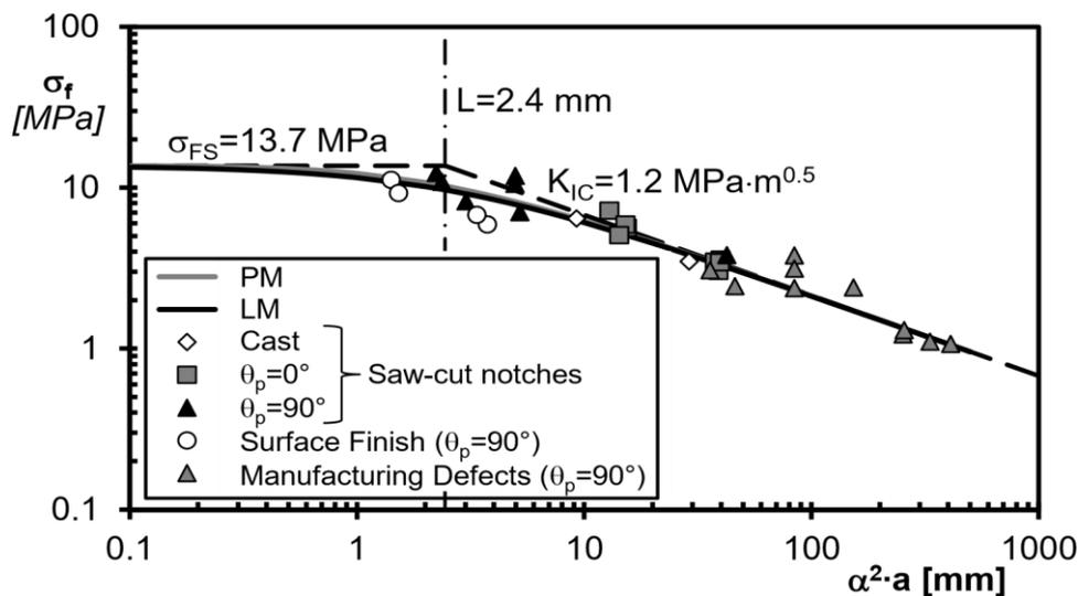
**Figure 1.** Accuracy of the TCD in modelling the detrimental effect of cracks and defects in 3D-printed concrete loaded in three-point bending.
