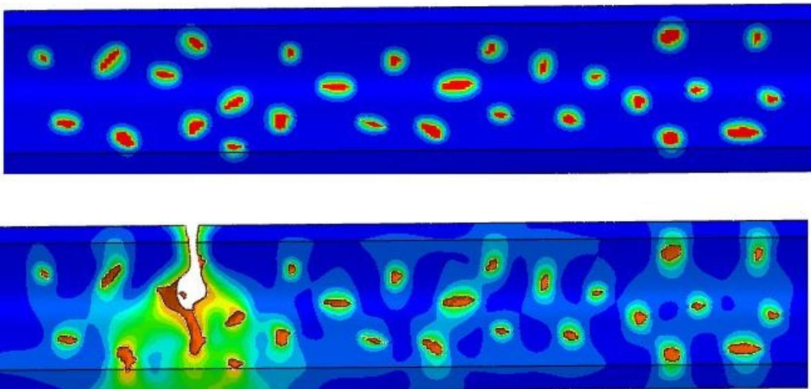
**Figure 1** – Evolution of damage in a pipeline. The corrosion pits, measured with in-line inspection, are introduced in the model by prescribing the initial value of the phase field.
