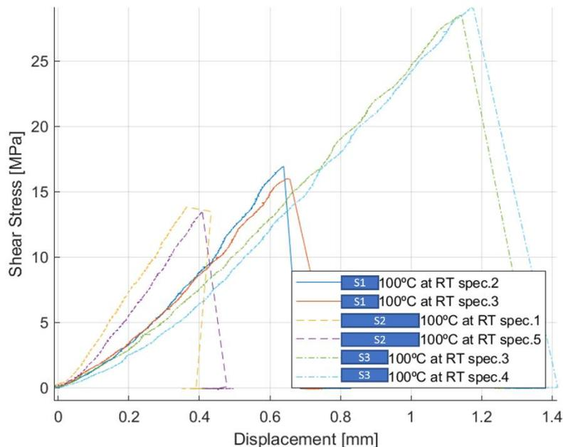
**Figure 1** – Shear stress vs. displacement of 3 CTC copper joints cured at 100°C for 80h
