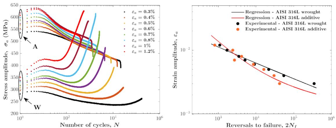
**Figure 1** - Cyclic stress response and strain-life curves for wrought (W) and L-PBF (A) AISI 316L stainless steel.
