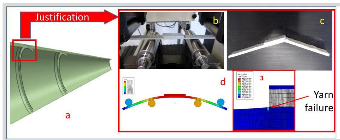
**Figure 1** – Illustration of (a) the stiffened CMC exhaust cone, (b) the four-point bending test on bonded CMC joints, (c) the fracture of the specimen and (d) the associated simulation with damage models
