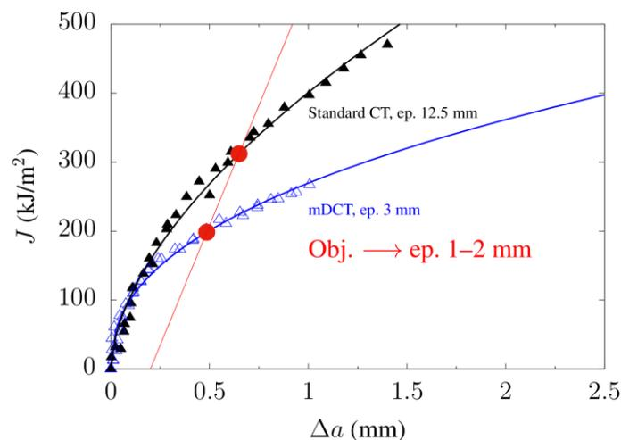
**Figure 1** -  $J$ - $\Delta a$  crack propagation curves for standard CT and sub-size mDCT specimens.
