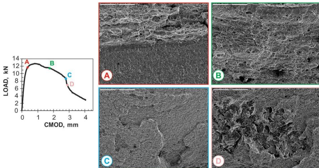
**Figure 1** - Load vs. CMOD curve for HAZ tested at  $-40\text{ }^{\circ}\text{C}$
