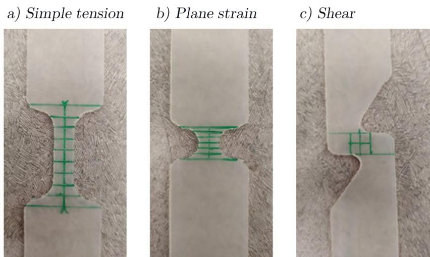
**Figure 1.** Different specimen geometries a) Simple tension b) Plane strain c) Shear
