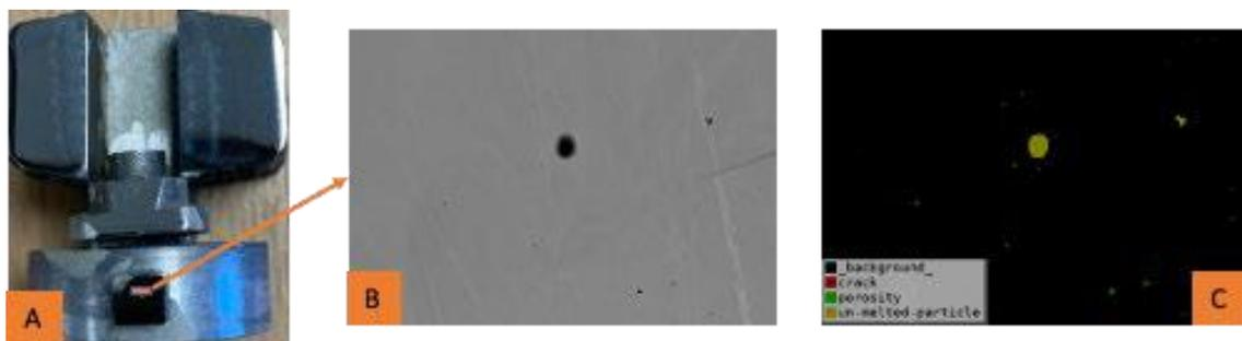
**Figure 1** – A) Metallographically polished 316L steel SLM and DED samples B) Example micrographs with different types of defects C) Masked micrographs used for training the neural network models
