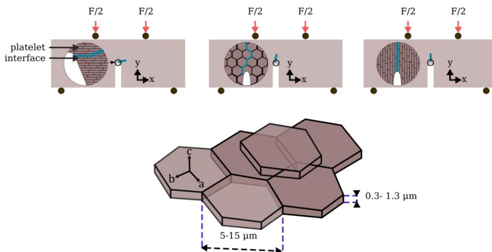
Figure 1 - fc-NLA with three different platelet orientations. On the left, the extensively studied configuration showing intensive crack deviation. In the middle and on the right, the two reference configurations under study.
