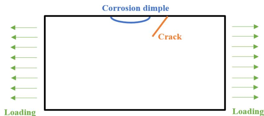
**Figure 1** – Scheme of the specimen with a crack propagating near a corrosion dimple
