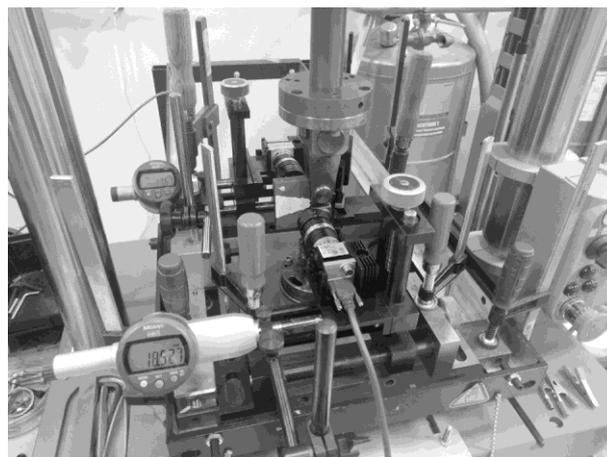
**Figure 1** – Fracture mechanical fatigue testing setup for PLA CT specimen
