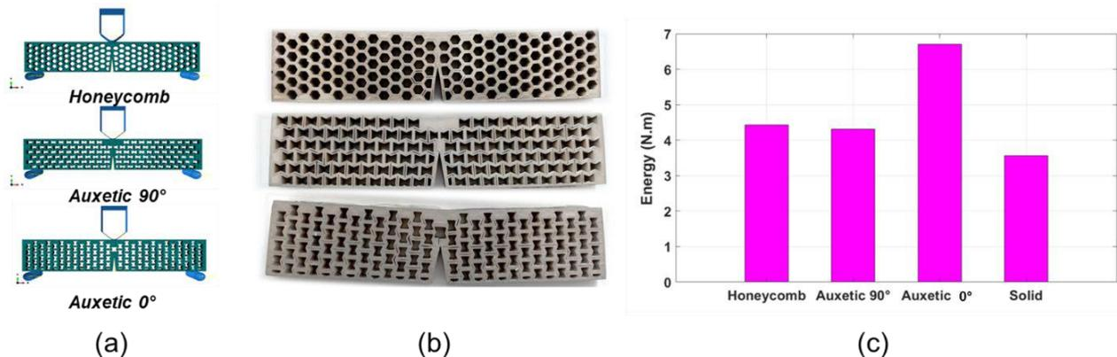
**Figure 1** – (a) Specimens geometries – (b) Damage observation (c) Experimental material toughness
