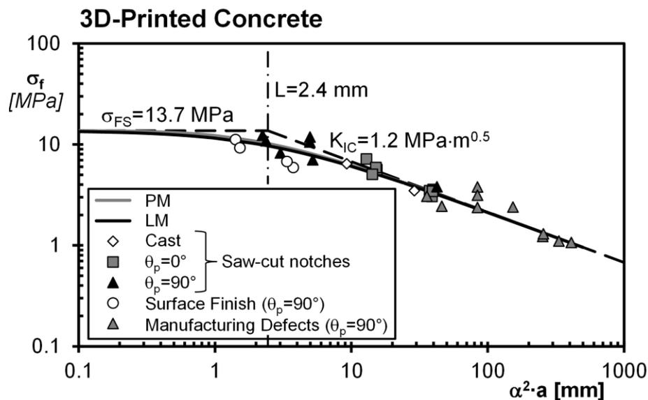
**Figure 1** - Accuracy of the TCD in modelling the detrimental effect of cracks and defects in 3D-printed concrete loaded in three-point bending.
