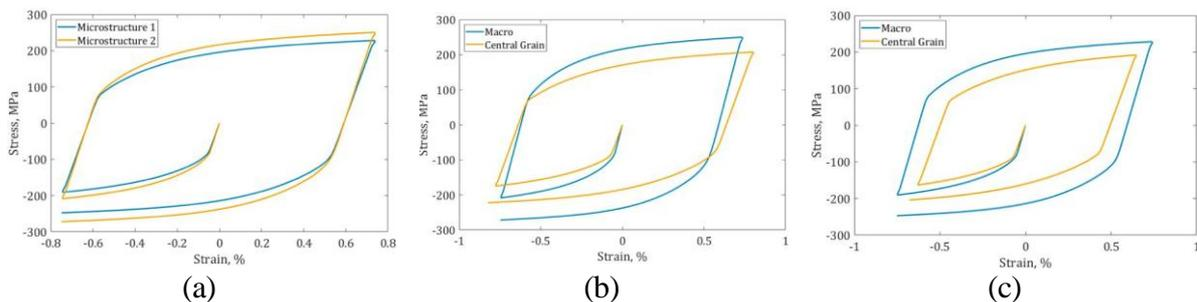
Figure 2- Comparison of the similar microstructure response with two different central grain orientation (a) macromechanical response of the two microstructure (b) macromechanical and central grain micromechanical response of microstructure 1 with a soft central grain (c) macromechanical and central grain micromechanical response of microstructure with a hard central grain.
