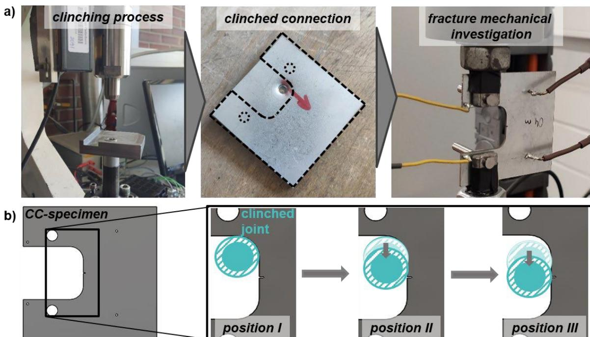
**Figure 1** – Illustration of the clinching process, the clinched connection and the fracture mechanical investigation (a), different positions of the clinched joint (b)
