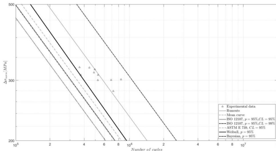
**Figure 1** - Comparison of the  $p_s = 5\%$  P-S-N curves from different methodologies for the hot-spot stress case.
