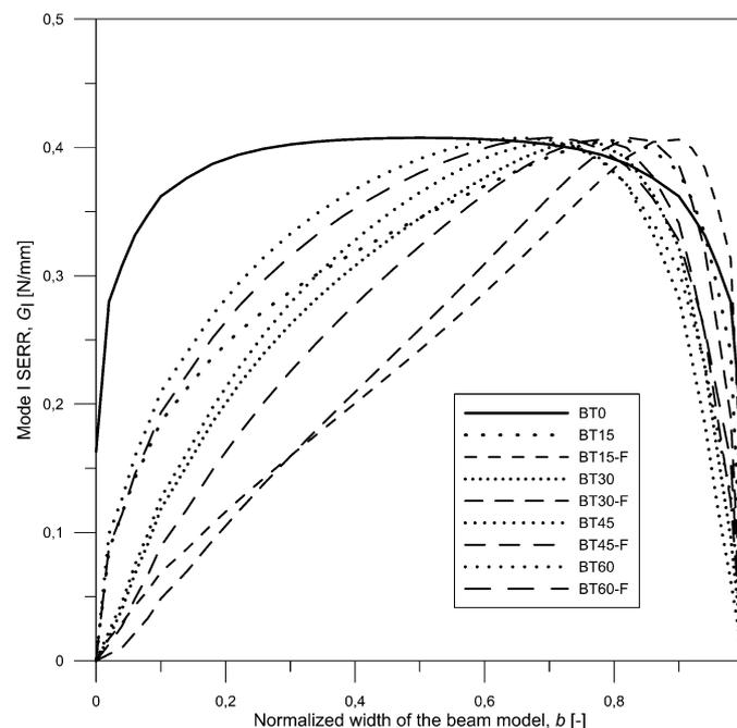
**Figure 1** – Mode I SERR distributions along delamination front in bending-twisting coupled laminate beam model
