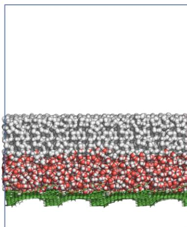
**Figure 1** – Ice adhesion on a substrate via a quasi-liquid water layer
