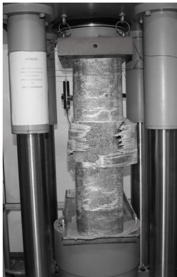
**Figure 1** - Failure of GFRP on a reinforced concrete square column
