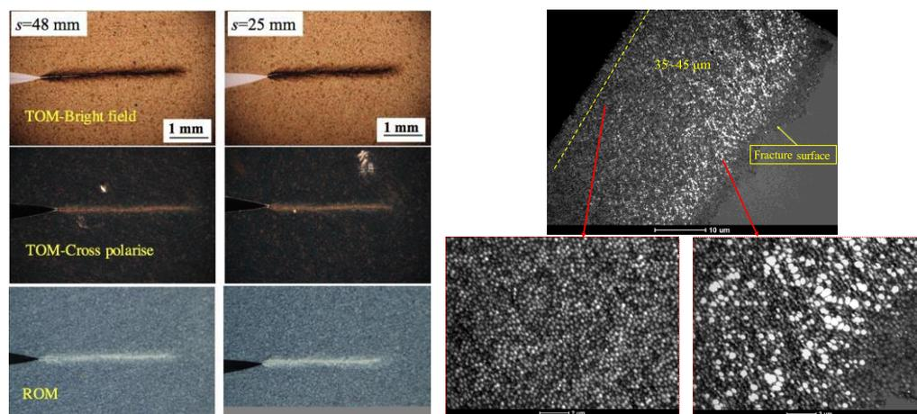
**Figure 1** - Microscopy images of fractured 3PB specimens; (a) Optical microscopy images of PDZ, (b) TEM images of FPZ.
