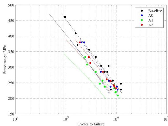
**Figure 1** – Wöhler curves for the baseline, A0, A1, and A2 process parameters set
