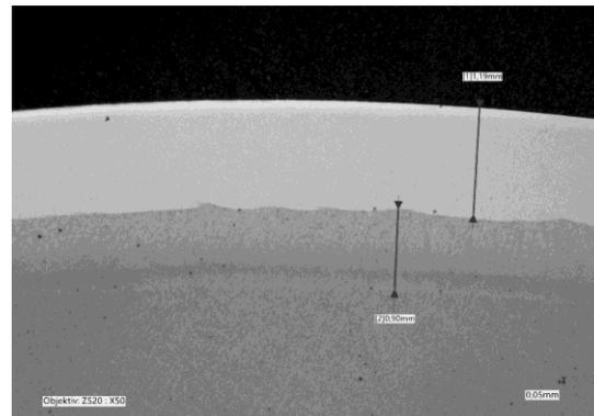
**Figure 2** - Example of detail of a 50× zoomed interface made from a structural steel with a hard chrome layer.
