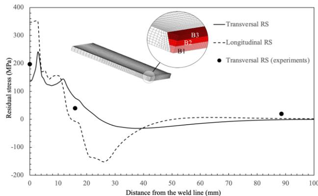
**Figure 1** – Residual stress: comparison between experimental and numerical results.
