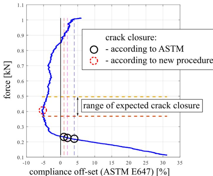
**Figure 1** – force-compliance record for evaluation of crack closure, herein standard ASTM E647 leads to underestimation of crack closure level
