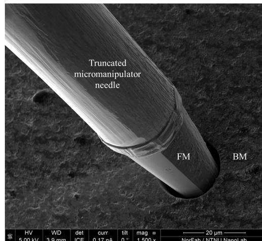
**Figure 1** – Microscale welding operation in a Focused Ion Beam (FIB) microscope: the Filler Metal (FM) is fed inside a hole drilled in the Base Metal (BM) by means of the FIB micromanipulator needle
