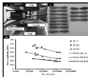
**Figure 2** – S-N Curve at different R-Ratios
