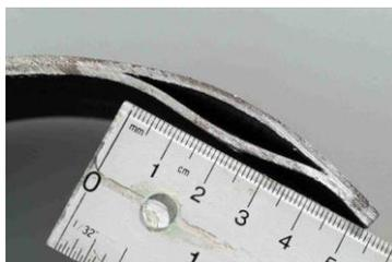
**Fig. 2a. Hydrogen Blister in NPS 6 Sour Gas Pipeline**
