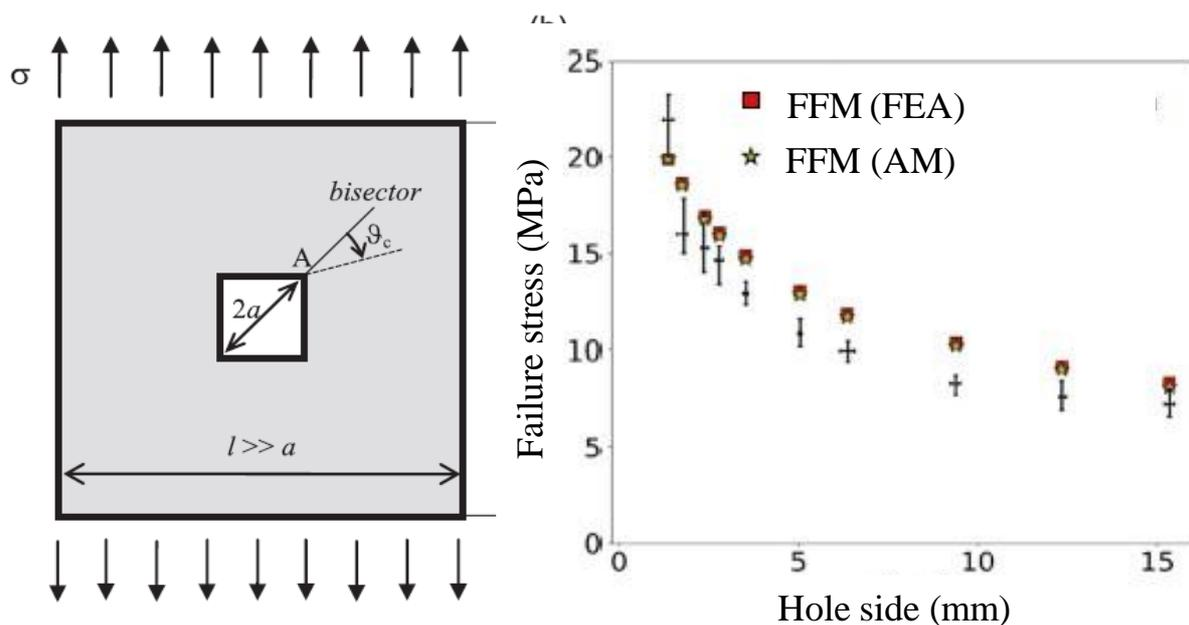
Figure 1 - Square holed plates and comparison between experimental and FFM results.
