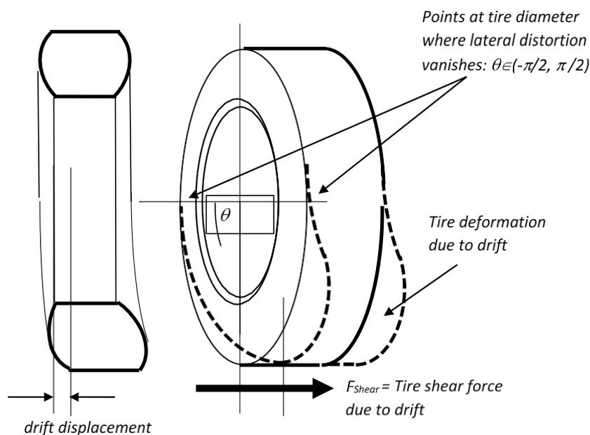
**Figure 1** – Tire distortion by lateral force due to cornering.
