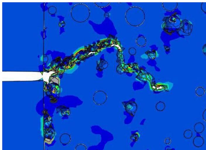
**Figure 1** – Probabilistic FEM analysis of crack propagation through the microstructure
