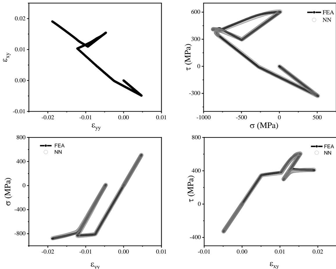
**Figure 1** – Stress-strain behaviour of the material during combined complex loading and corresponding neural network predictions
