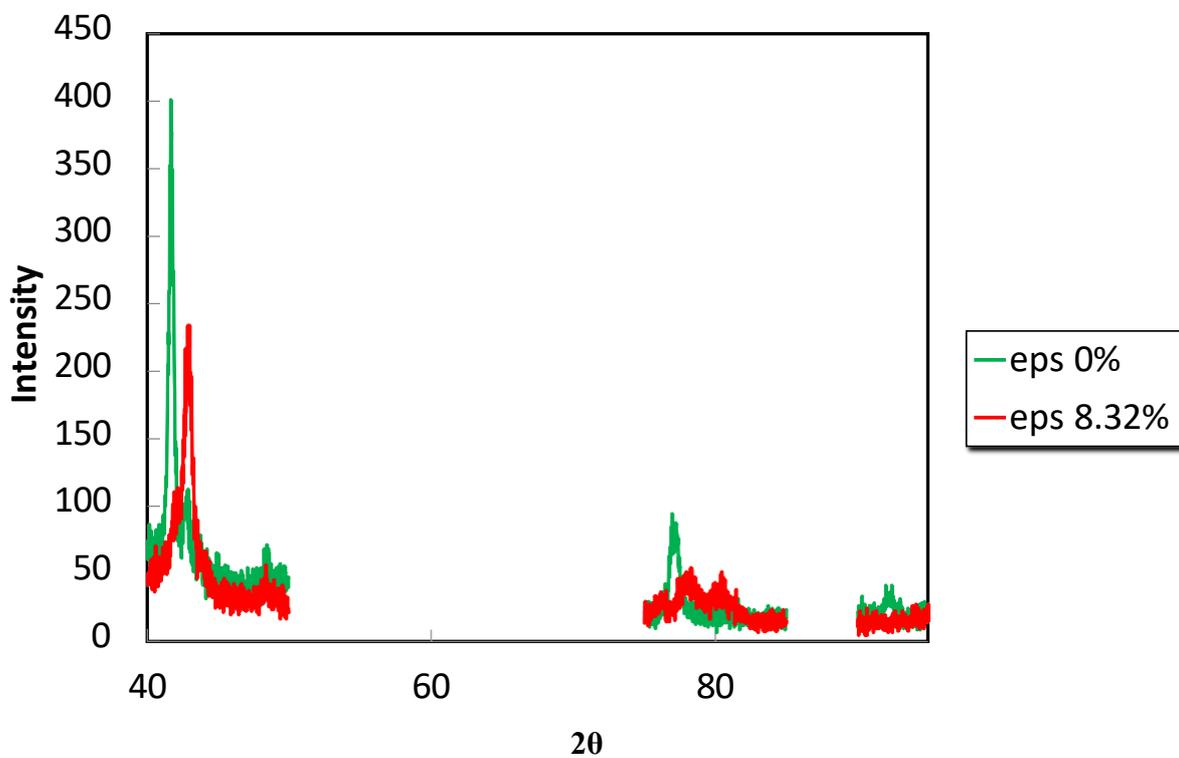
*Figure 1 – Austenite and Martensite diffraction spectra*
