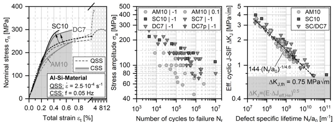
**Figure 1** – Uniform fatigue damage tolerance law based on batch-specific (a) CSS curves in comparison to QSS curves, (b) S-N diagram according to Woehler including defect-, plasticity and R-related scatter and (c) K-N diagram according to Shiozawa using the effective cyclic J-Integral at local fracture-initiating defect.
