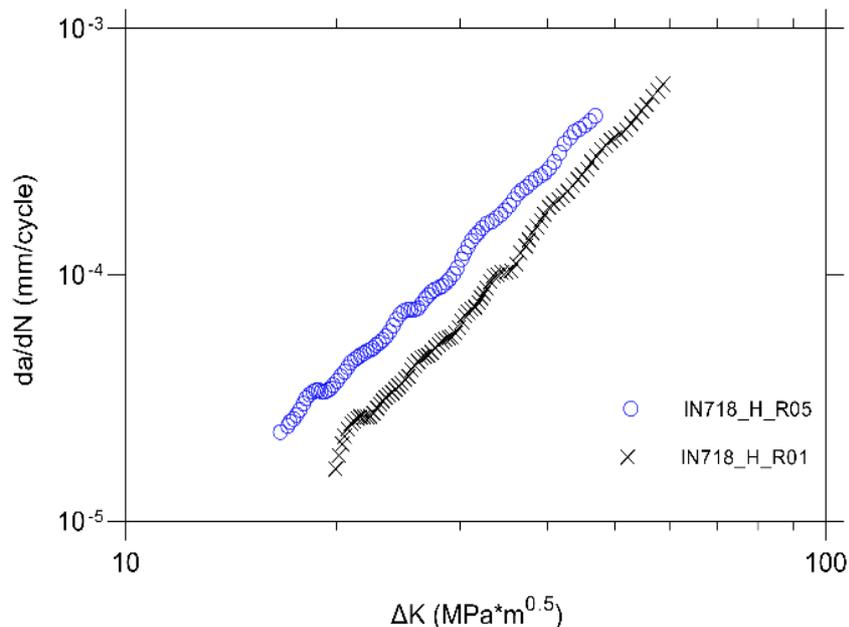
**Figure 1** – Fatigue crack growth rate for IN718 after HIP for R-0.1 and R-0.5
