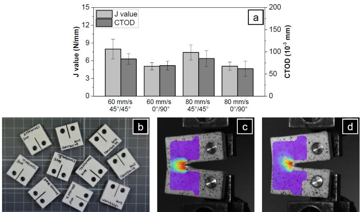
**Figure 1** – Fracture mechanics parameters for ABS at impact loading as a function of the processing parameters (a); fracture mechanics tests (0°/90° (c) and 45°/45° (d)) on small CT specimens (b) of ABS at quasi-static loading combined with strain field analysis
