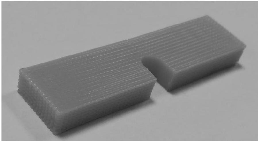
*Figure 1 – PLA SENB specimen containing a U-notch (radius = 2.0 mm)*
