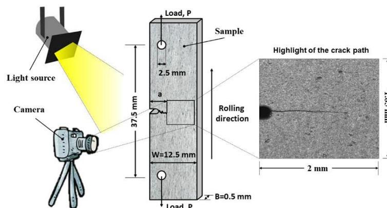
**Figure 1:** Eccentrically loaded single edge crack (ESE) specimen and experimental setup
