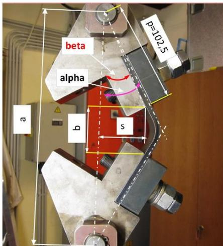
Figure 1 - Apparatus for loading of bended billet
