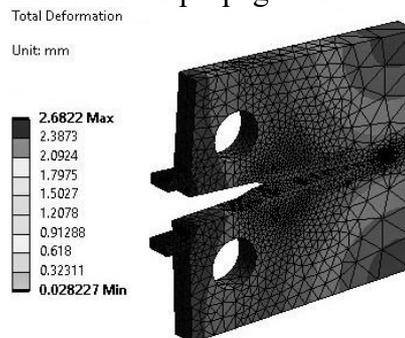
*Figure 1 – Compact tension test piece finite element model*
