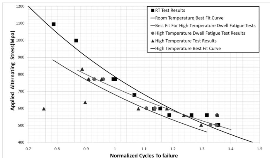
Figure 1 –S-N curve of Inconel 718 after Rotating Bending fatigue tests
