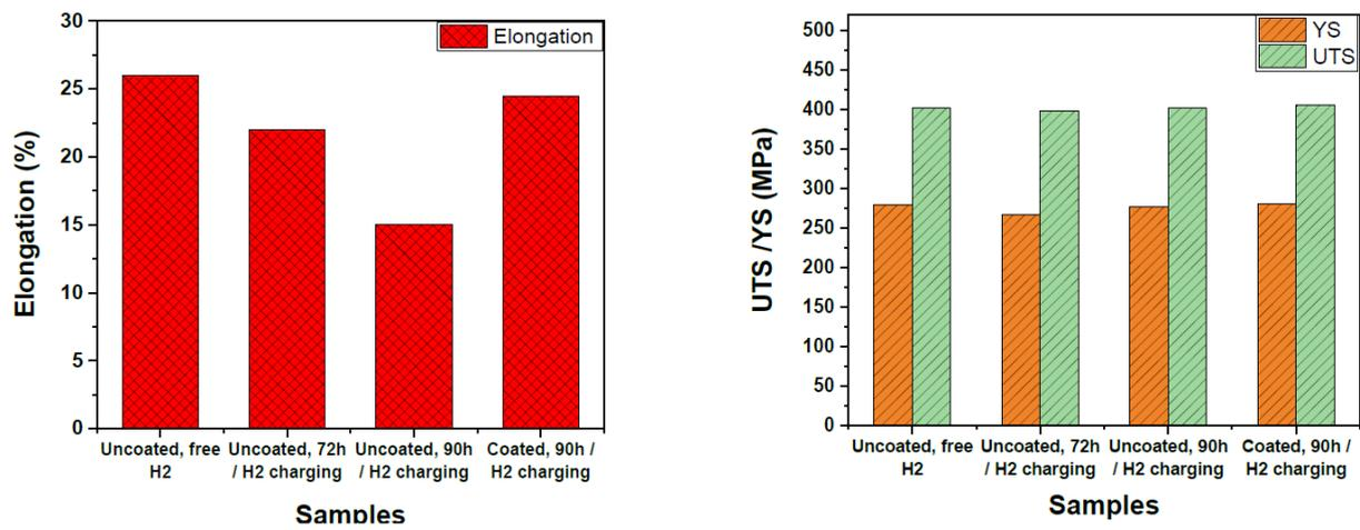
**Figure 1:** Tensile properties of uncoated specimens tested at different pre-charging time and coated specimen pre-charged at 90 hours.
