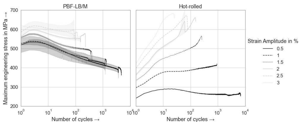
**Figure 1** – Maximum engineering stress vs. number of cycles for both the PBF-LB/M-process and the hot-rolling process
