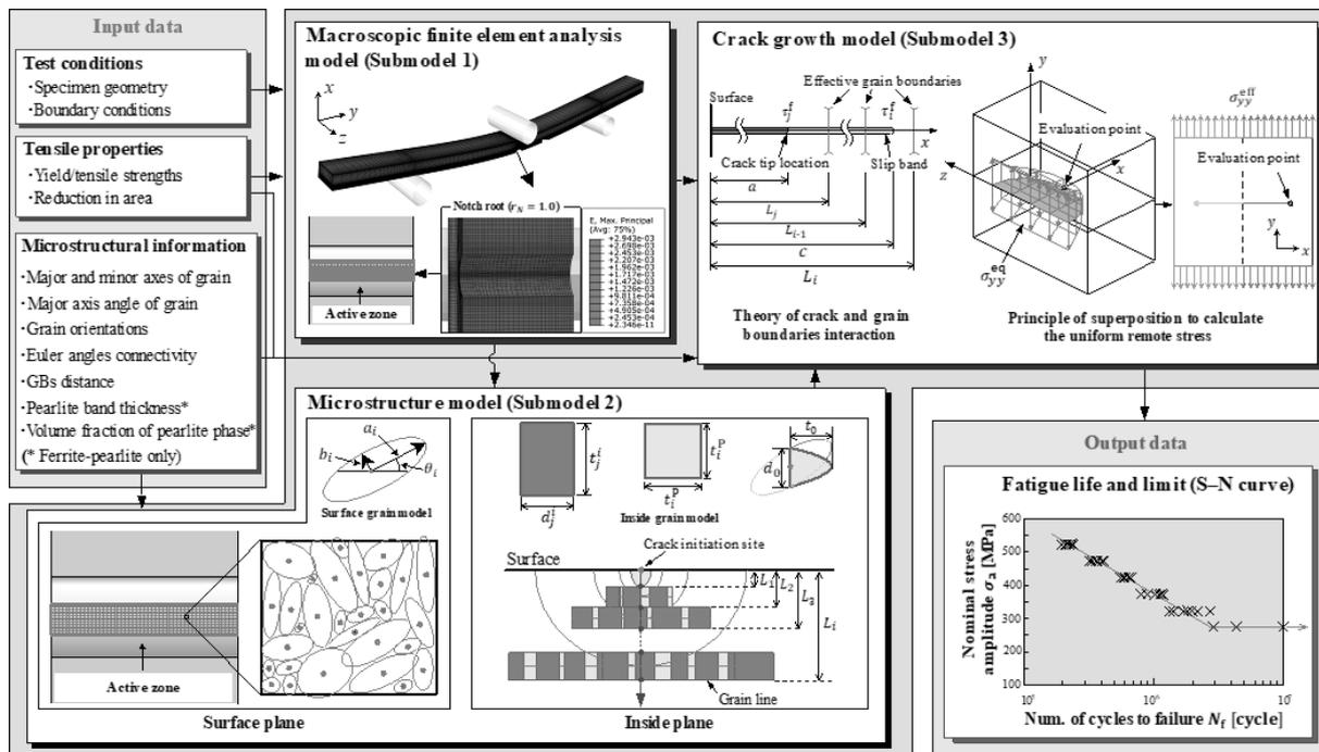
Figure 1 - . Outline of proposed multiscale model for predicting the fatigue strengths of steel
