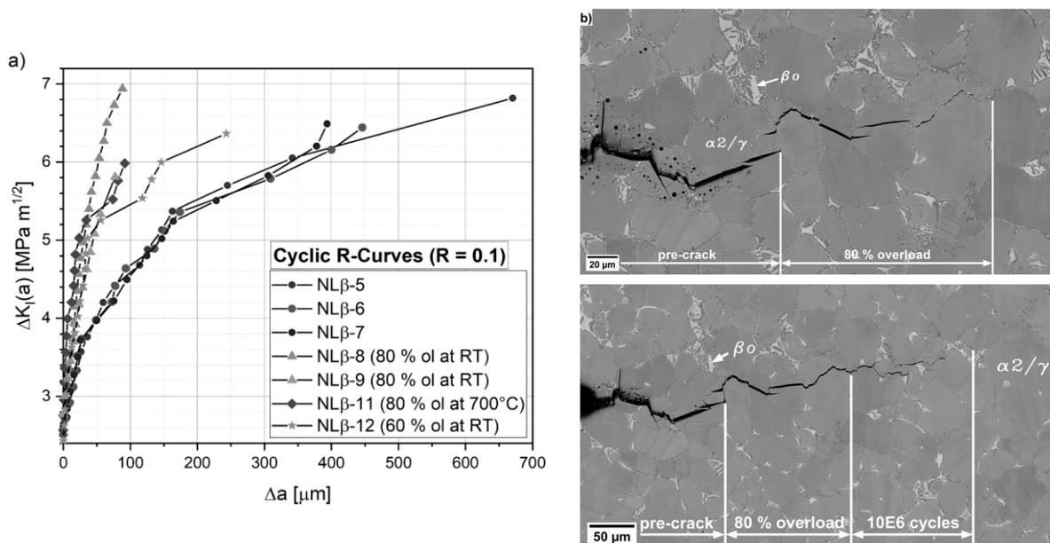
**Figure 1** – a) Cyclic crack resistance curves (R-curves) of the threshold  $\Delta K_{th}$  at a load ratio of  $R = 0.1$ , b) SEM crack path analysis of an overload experiment
