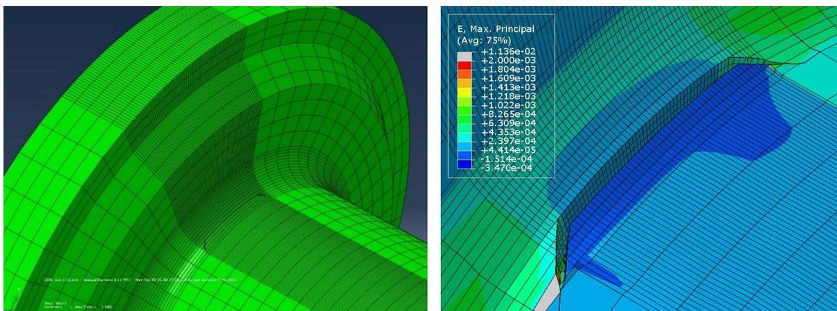
**Figure 1** - Position of the initial fatigue crack on one of the iterations during simulation
