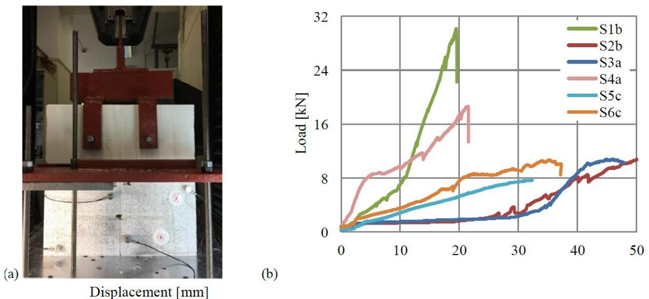
Figure 1 – (a) The experimental set-up. (b) Typical load-displacement curves.
