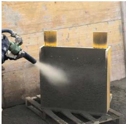
**Figure 1** - Mixture stream projected at high velocity onto a surface.
