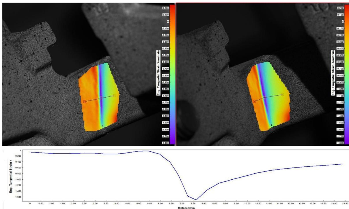
Figure 1 Notched component X direction strain distribution
