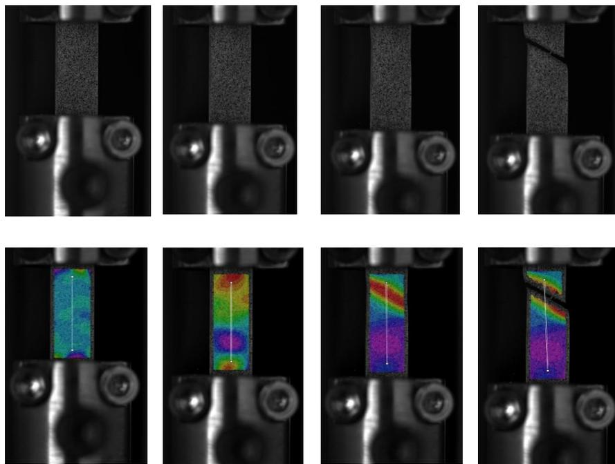
*Figure 1 – Digital Image Correlation strain measurements in high strain-rate tensile testing of a metal additive manufacturing specimen*
