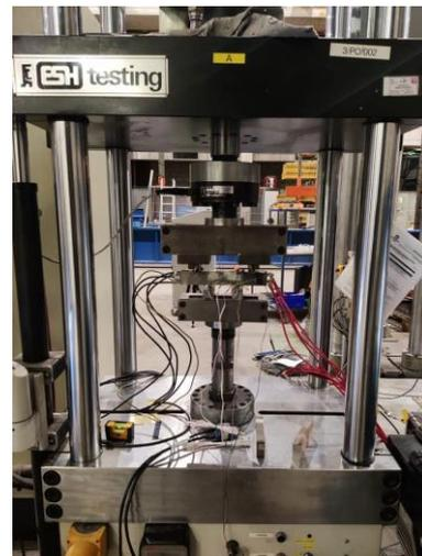
*Figure 2 – Test setup for fatigue four point bending.*
