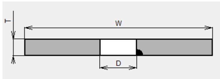
Figure 1 – Single corner crack at hole
