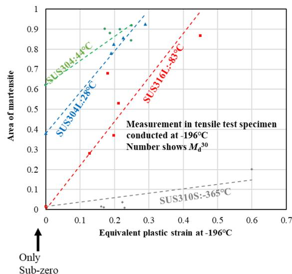
**Figure 1** – Relation between plastic strain amount and martensite transformation when mono-axis tension
