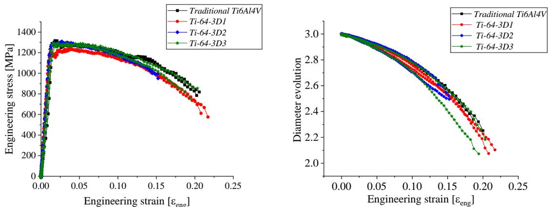
Figure 1: Engineering stress -strain response and evolution of necking diameter for traditional and additively manufactured Ti6Al4V.
