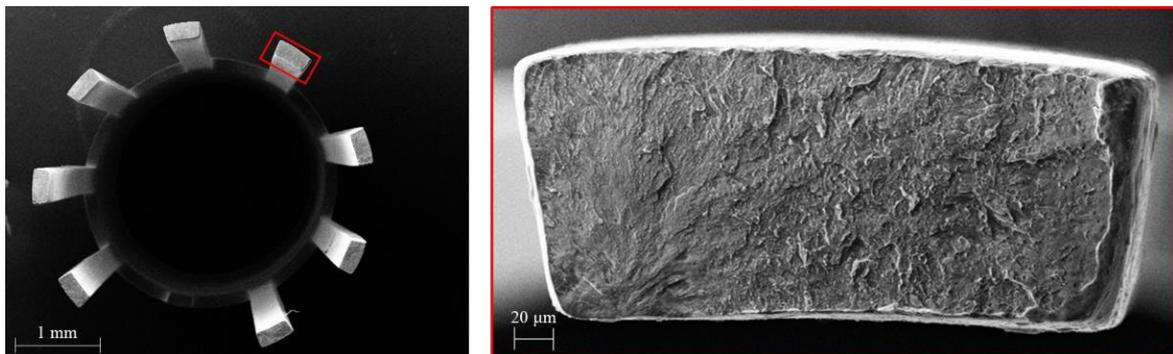
**Figure 1** – SEM acquisitions of one Ni-Ti multi-wires sample, with a focus on the fracture surface of a single wire
