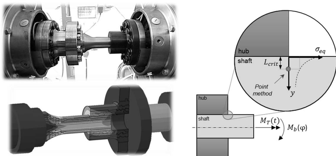
**Figure 1** – Determination of critical distance for multiaxially loaded shrink-fit connections based on experimental investigations
