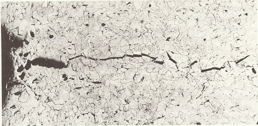
Figure 8.9 Change in fracture mechanism from fibrous to cleavage as a crack grows (mild steel, room temperature) ( \times 42 )
